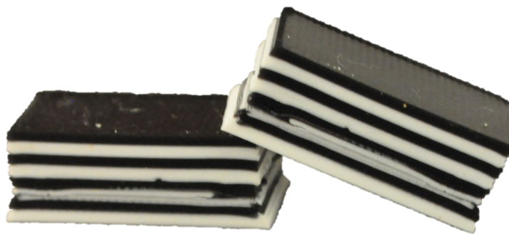
Figure 4.7: Image showing a printed scaffold, using the multi-tip method, the two materials used were white and black silicone, and represents the schematic in Figure 4.6a.
