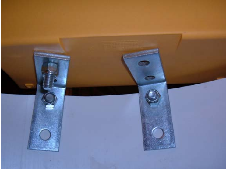
Figure 13: L-brackets mounted to toolbox and PVC tubing support
