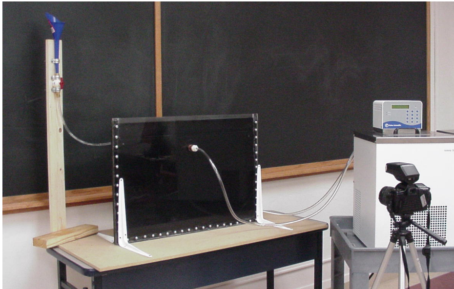
Figure 6.9 Hele-Shaw flow visualization setup.
