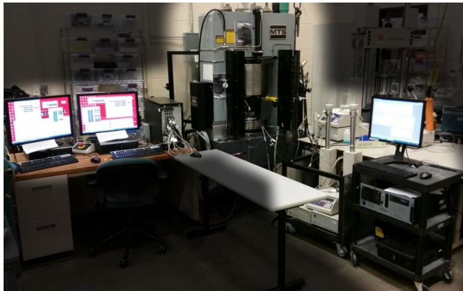
Figure 3. Multistage Triaxial Experimental Setup with 315 Load Frame
