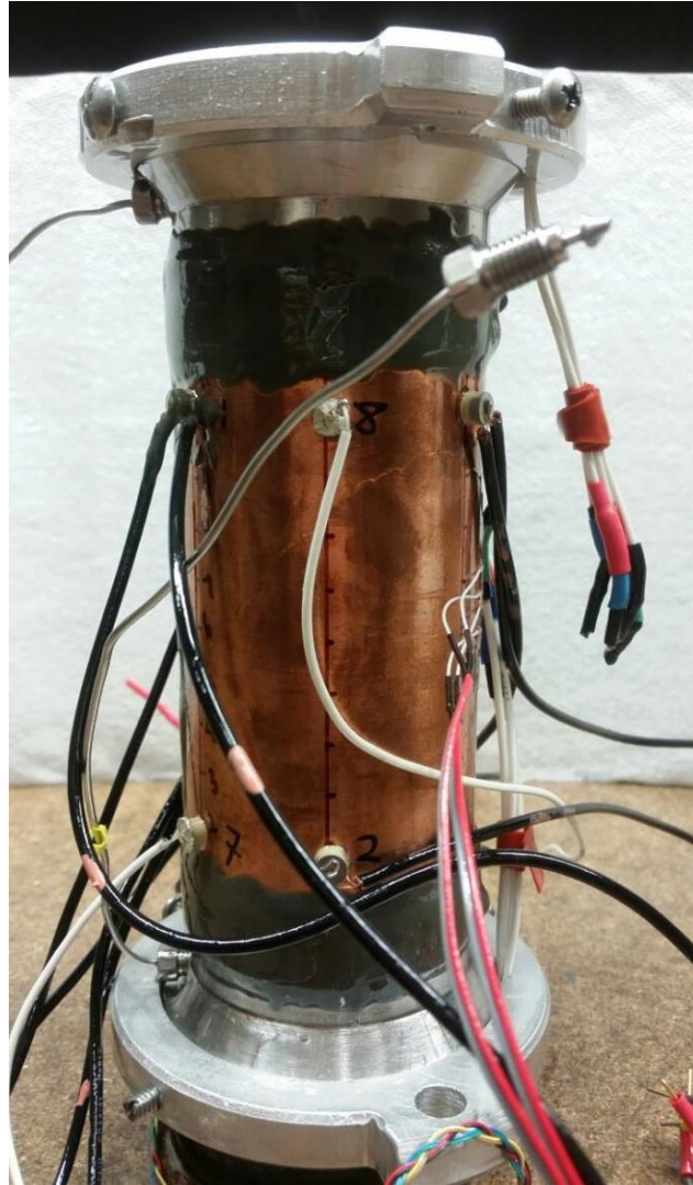
Figure 47. Sample B with Attached Acoustic Emission Crystals
