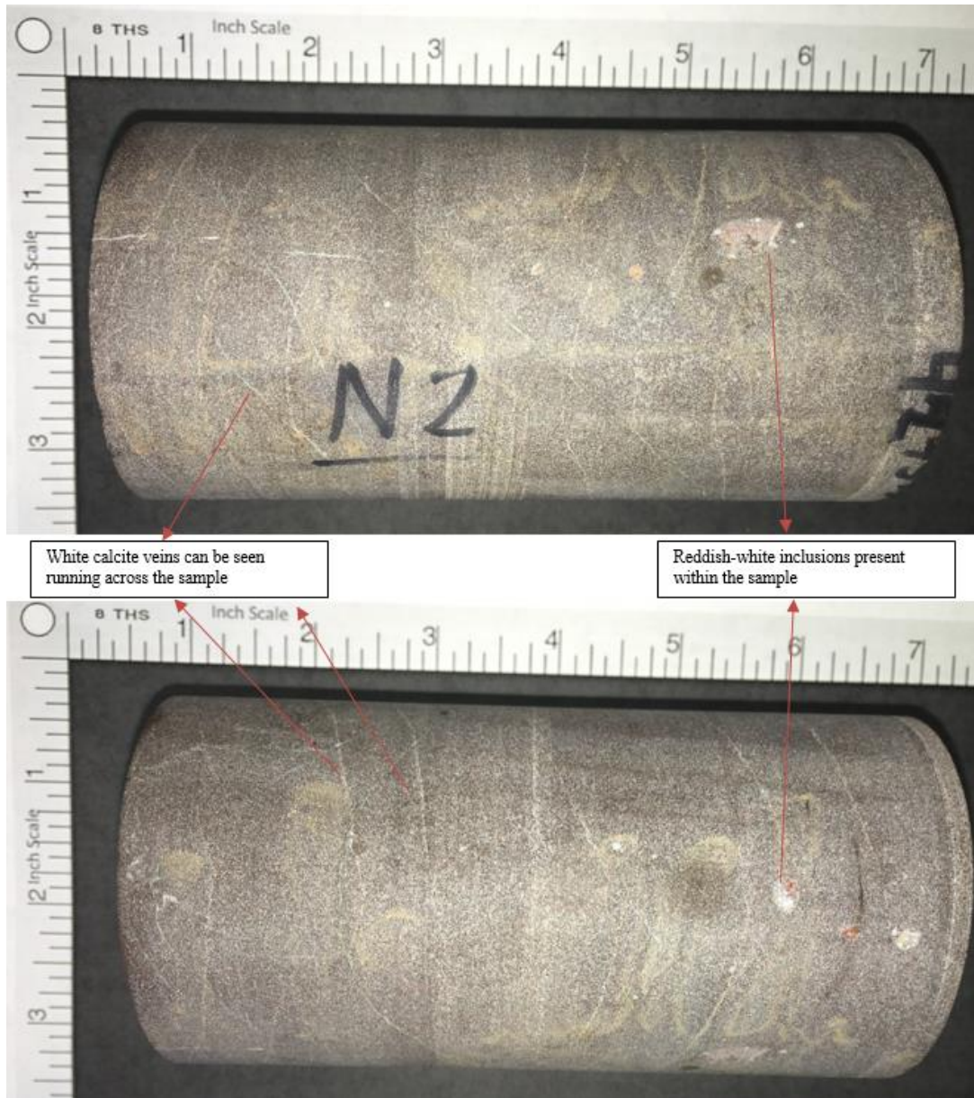
Figure 37. Sample B Cut and Polished Before Test
