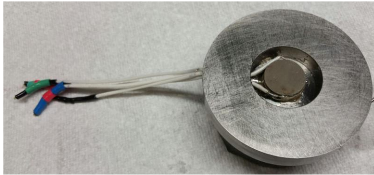
Figure 8. Velocity Measurement Crystals Embedded in Platens
