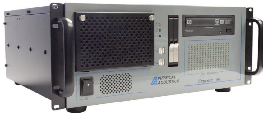
Figure 7. MISTRAS Industrial Express large PCI Express AE chassis
