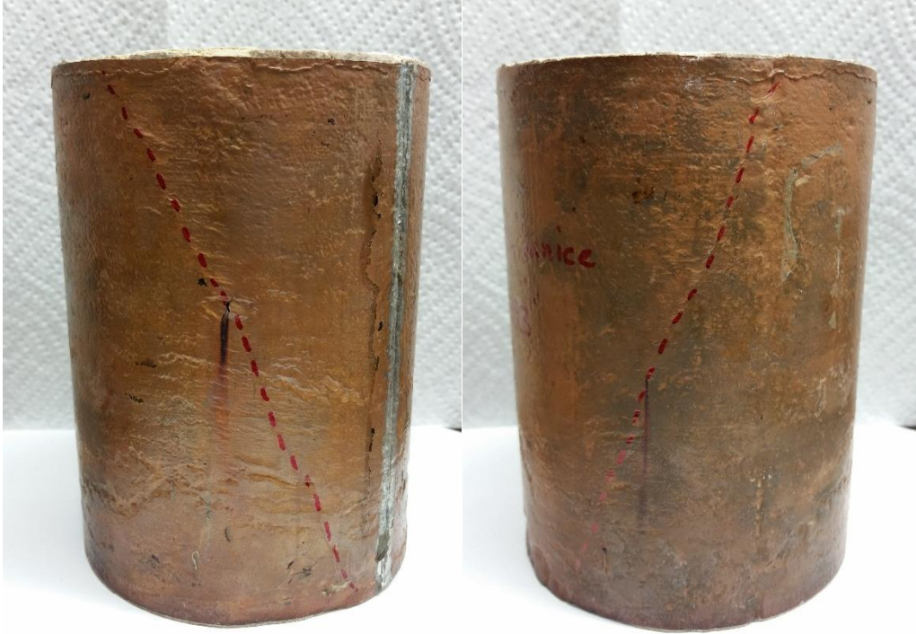
Figure 59. Sample C after Failure (Two Views)
