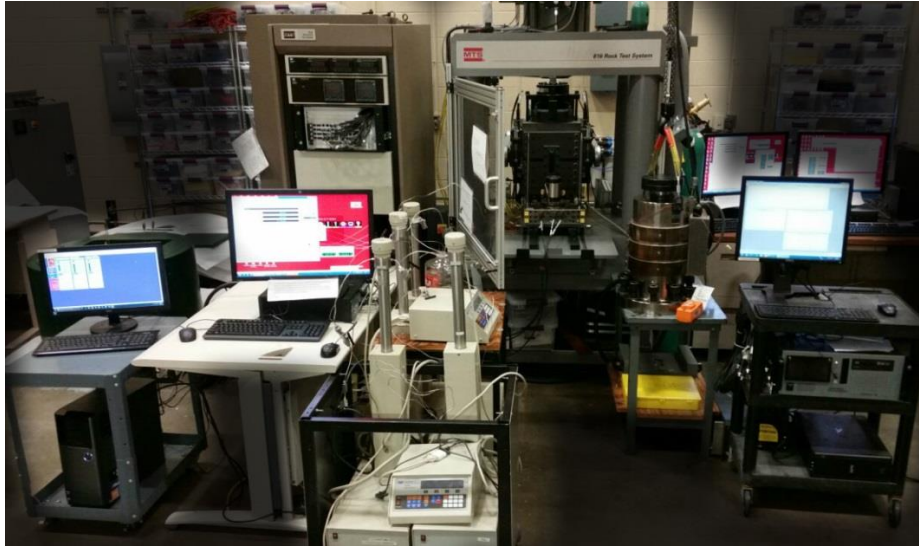
Figure 2. Multistage Triaxial Experimental Setup with MTS 816 Rock Mechanics Test System
