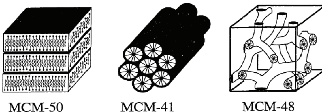
Figure 1.6. Schematic of the M41S materials: MCM-50 (layered), MCM-41 (hexagonal) and MCM-48 (Cubic).
