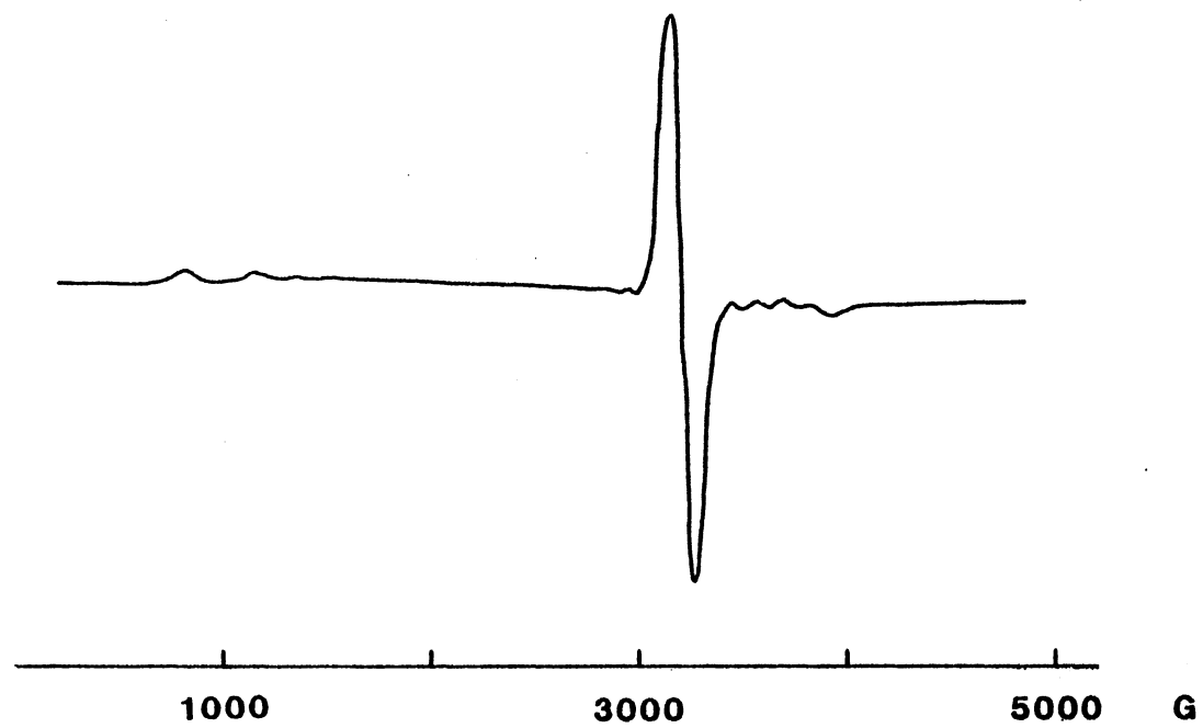
Figure 3. ESR spectrum of LiNbO 3 taken at 77 K after an x-irradiation at 77 K
