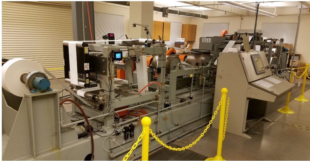
Figure 1 – Photo of the Euclid Web Line. The unwind section is in the foreground.
