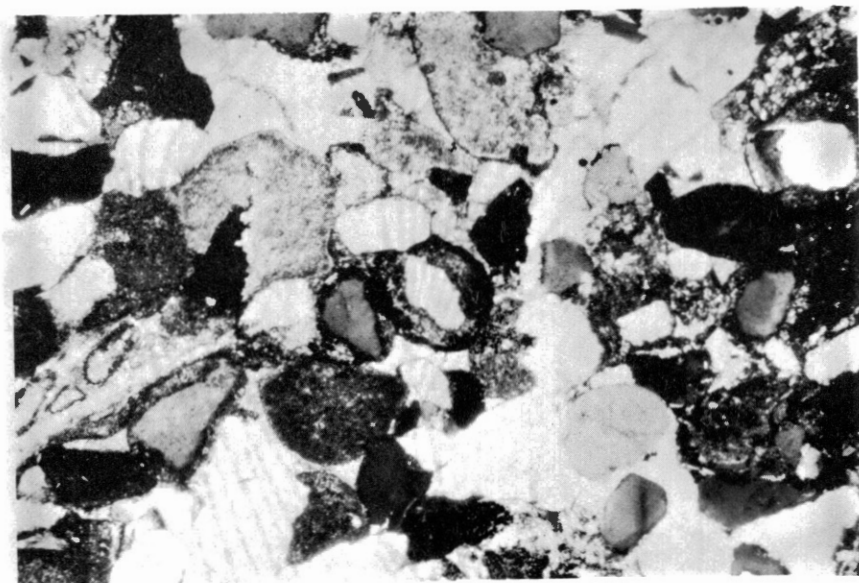
Fig. 41.-Tightly packed and cemented sandstone containing oolites with large quartz nuclei. Some quartz grains have corroded rims; others show overgrowths. Sandstone is massively bedded. Phillips Petroleum Company, Walters "J" No. 1, from depth of 10,317 feet. Crossed nicols X50.
