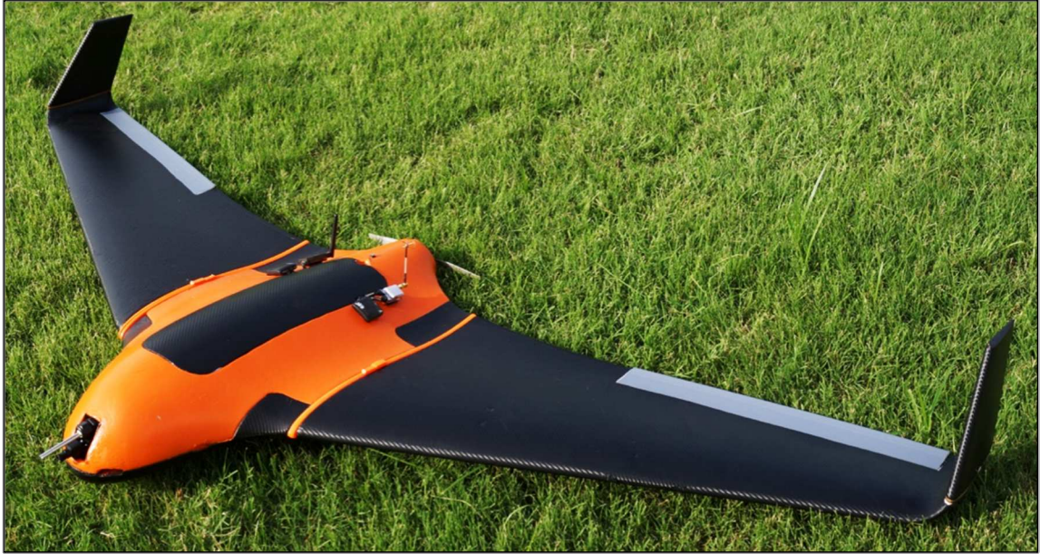
Figure 3 - OSU Sensorcraft, equipped with a small optical point chemical sensor.
