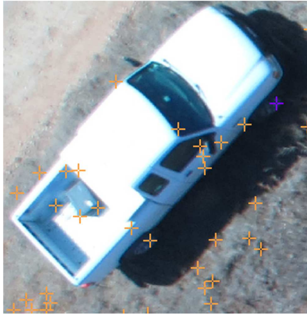
Figure 47 - an example of the available points for measuring the distance between the tires. The identical points on the front and back tires were selected.
