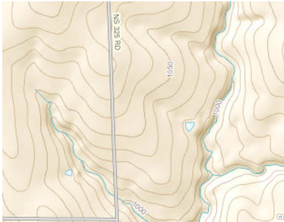
Figure 41 - USGS 30 meter DEM contour map (10 foot contour intervals) of the test plots
