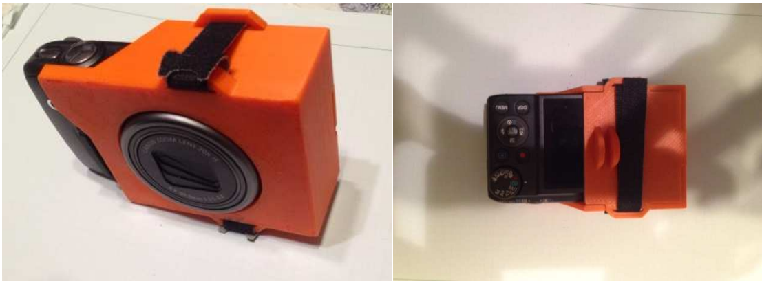
Figure 7 - Modified Canon SX260 HS camera with custom build aircraft mount.
