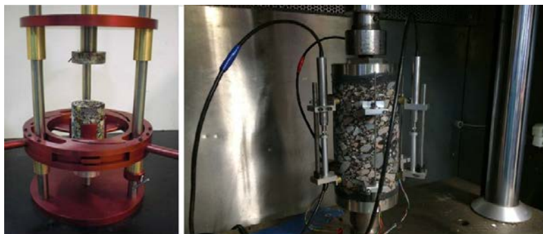
Figure 36 Uniaxial Fatigue Test Sample Gluing Process (left) and sample Setup inside Testing Chamber (right).
