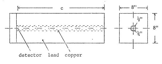
Figure 38. Collimator detail
