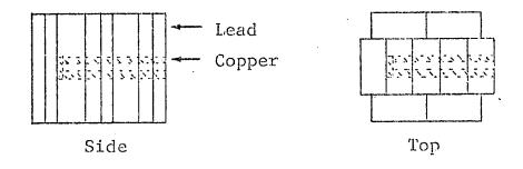
Figure 16. Detector collimator
