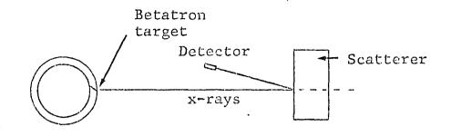
Figure 4. Experimental arrangement used by Sugiyama and Tomimasu.
