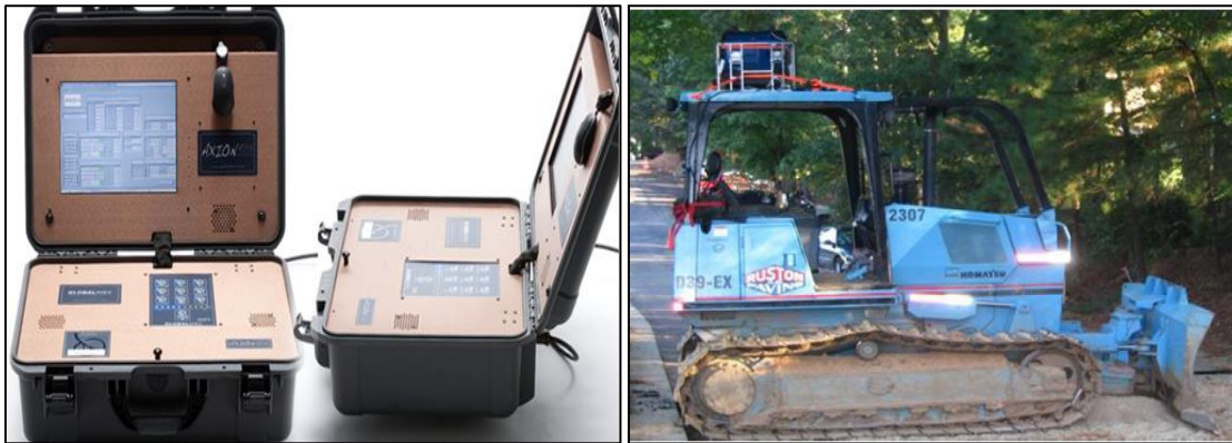
Figure 3.2. Installation of PEMS on HDD Equipment (Frey et al. , 2008)
