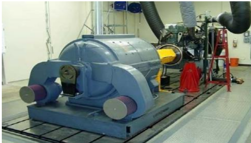
Figure 2.1. Engine Dynamometer (Mudgal, 2009)
