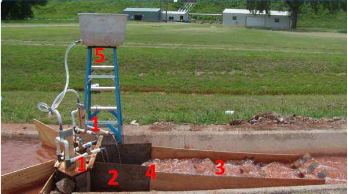
Figure 24. Prototype turbidity reduction system. (1) float valves for flocculant dosing, (2) metal cutthroat flume for flow measurement, (3) mixing structure, (4) hydraulic jump upstream of the mixing structure, and (5) flocculant tank.
