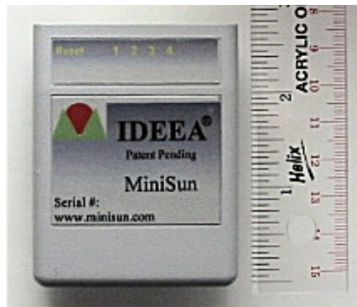
Figure 2.5. Intelligent Device for Energy Expenditure and Physical Activity.
