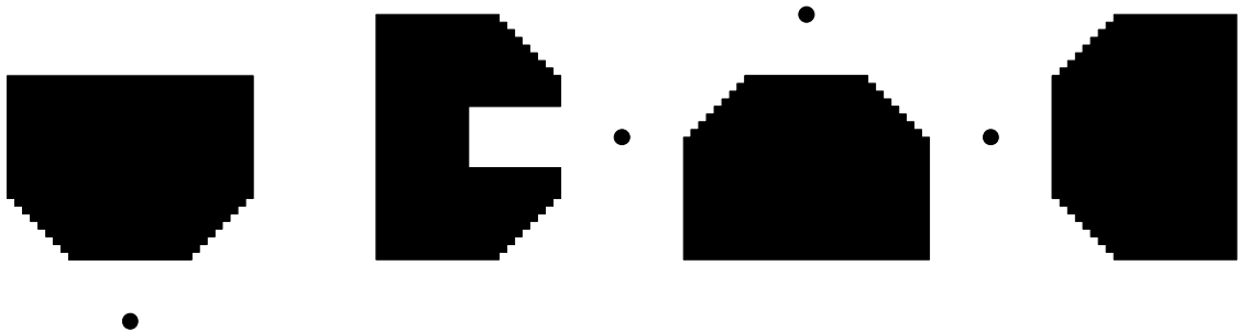
Figure 12. Binary volumetric model formed from each camera's view.
