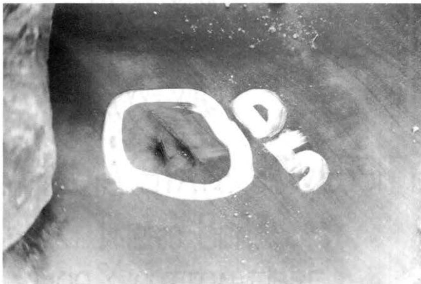
Figure 38. Cloth D, One and Two Inch Tears After 4.5 ft. Drop
