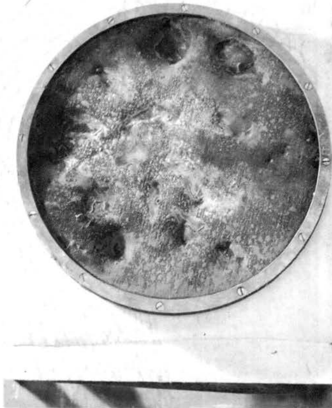
Figure 14. Cloth B After Completion of Test 5 (Underside of Cloth)
