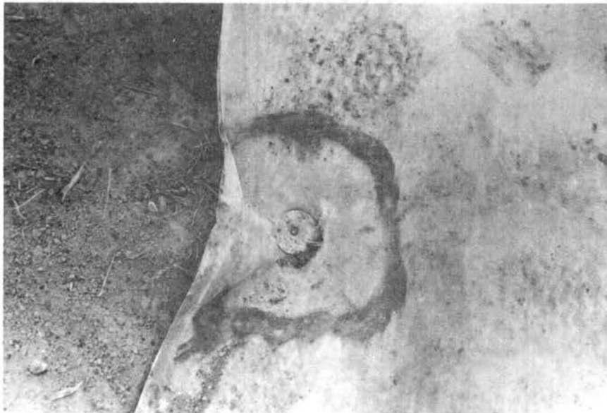
Figure 39. Cloth E, Tear Caused by Direct Hit of Stone on Securing Pin Washer
