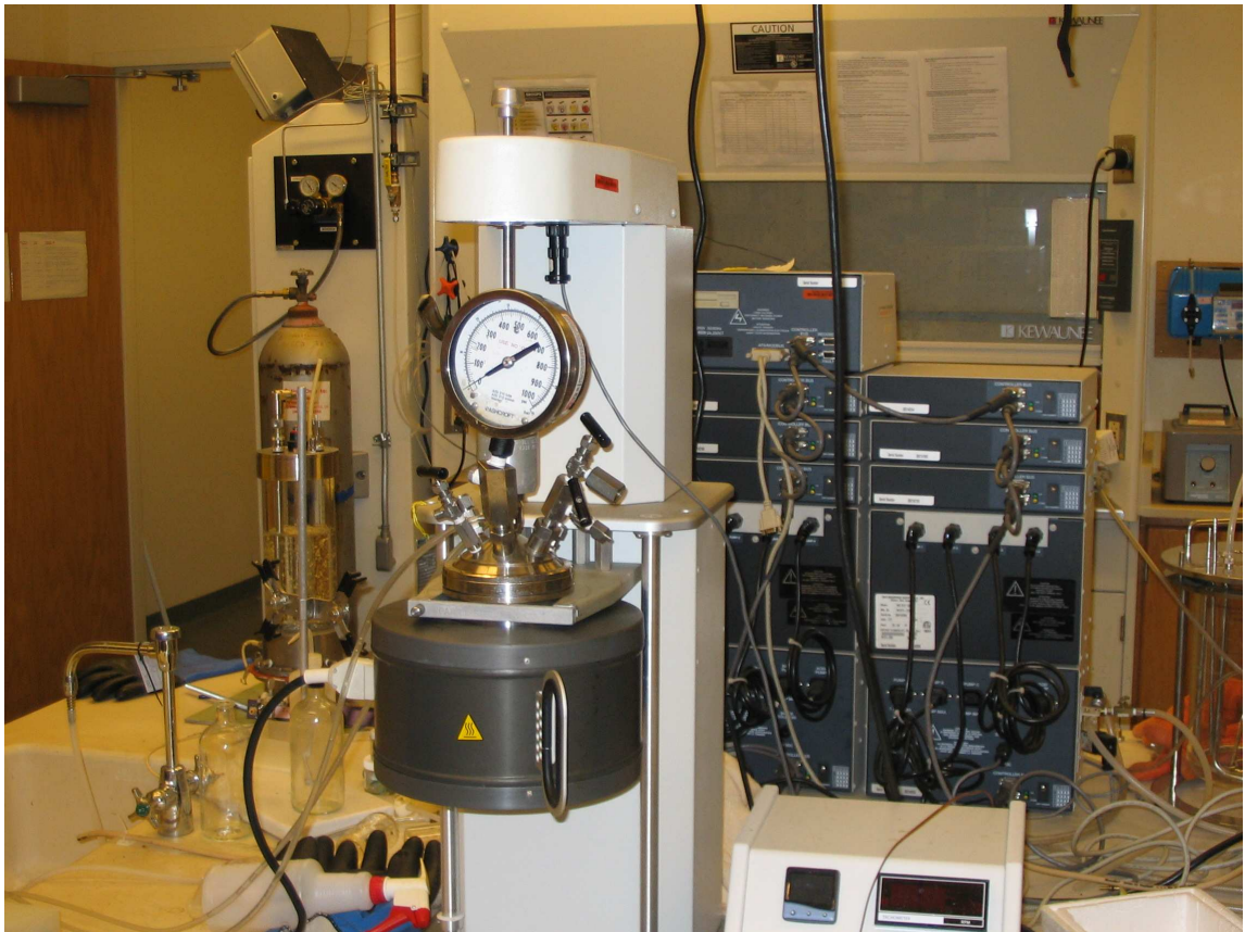
Figure 4.1 1-L Parr Pressure Reactor used for Hydrothermolysis of Switchgrass at 200 °C.
