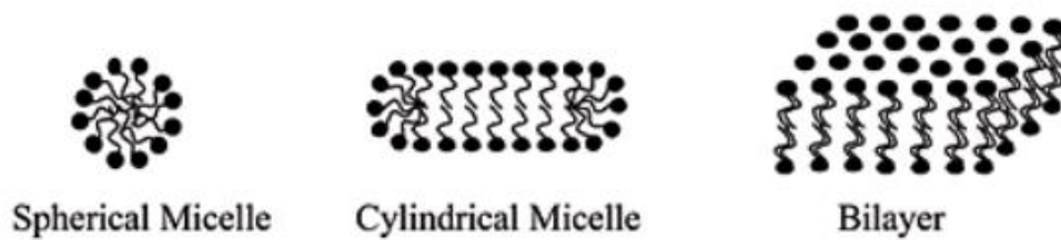
Figure. 3. Schematic Illustration of Three Main Types of Micelle Shapes (Som et al. 2012)
