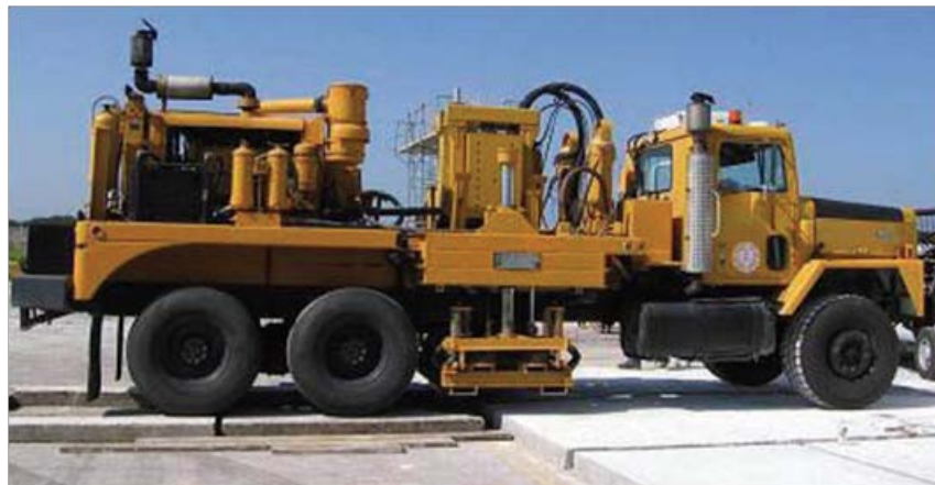
Figure 3.2: Field Testing Arrangement for super accelerated load testing.
