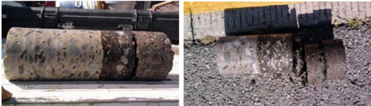
Figure 2.26 - Cores extracted on the oldest McAlester Overlay.
