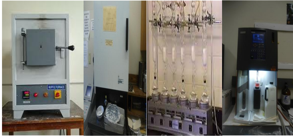
Fig 4. Proximate analysis instruments: from left to right, muffle furnace, forced air oven, Soxhlet extractor and Kjeldal equipment.
