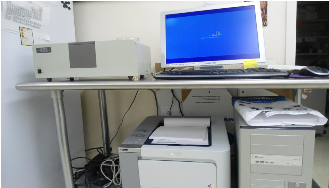
Fig 5. The spectrophotometer or Chromameter instrument used to measure the color of goat-meat sausage samples.
