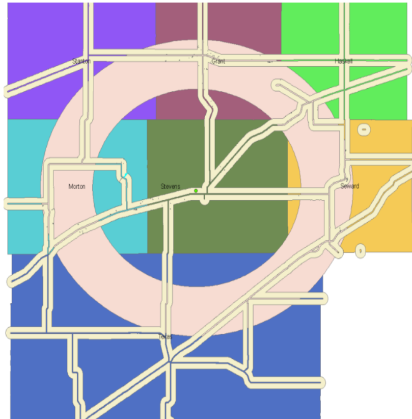
Figure 3.4. The buffer layer for road network and distance from biorefinery site for determining potential inventory sites
