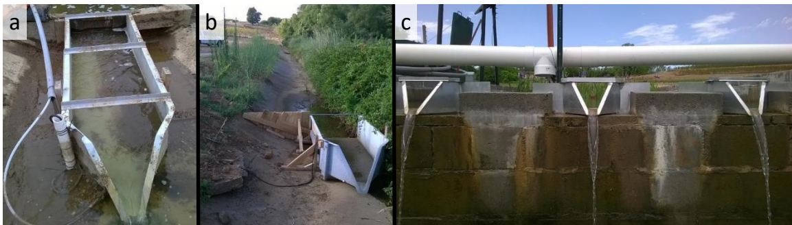
Figure 2.4 - Flumes used for flow measurement for the free-surface constructed wetland. a - H-flume measuring inflow. b - H-flume measuring flow in the main channel. c – Configuration of 3 H-flumes measuring outflow.
