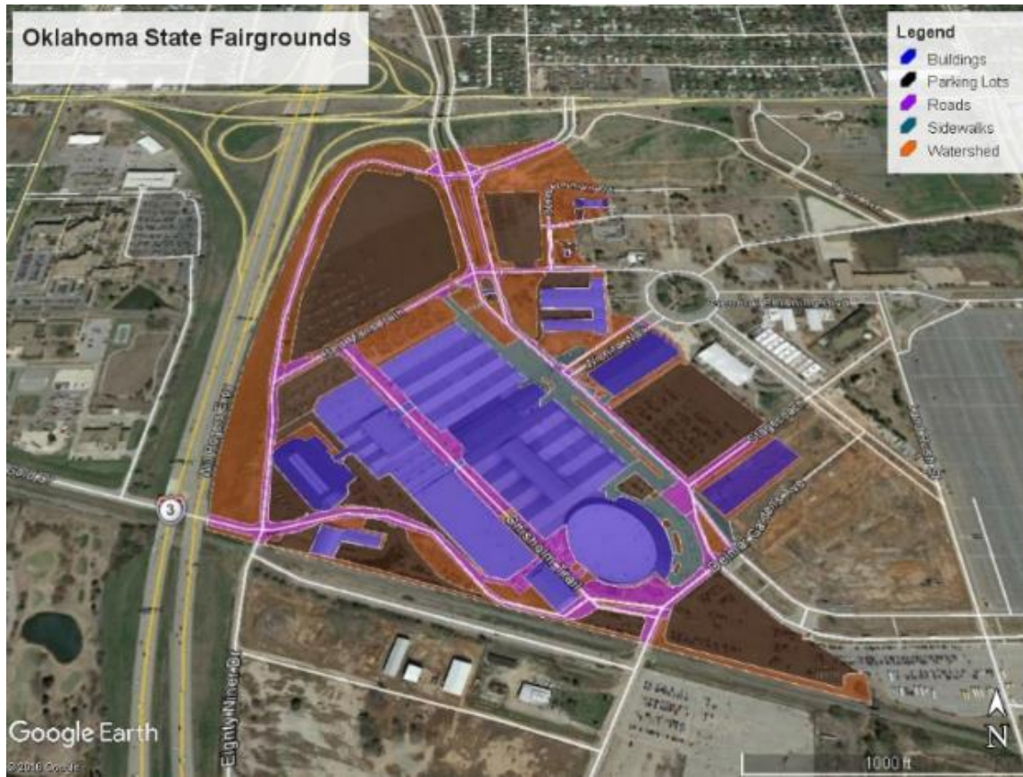
Figure 4.2 - Watershed delineation of State Fair Park in Oklahoma City, OK with land use highlighted. Building the Base Model. The first step in building the base model was to determine watershed characteristics of soil type, soil drainage rate, topography, and land cover. (Table 4.2). Site characteristics were determined both from the online database accessible in the SWC and prior knowledge of the site (Table 4.3). A precipitation gauge and weather station were chosen based on their proximity to the site and period of record. Both were at the same location (Will Rogers Airport, Oklahoma City, OK) which is approximately 5.3 miles from the site and had 36 years of historical data (1970-2006). After all watershed characteristics were input to the SWC, the baseline model was run and produced 25.1 inches of annual runoff from the average 34 inches of precipitation. The predevelopment runoff depth was determined by changing the land use to 90% meadow and 10% forest. This scenario produced 11.7 inches of annual runoff. Total runoff
