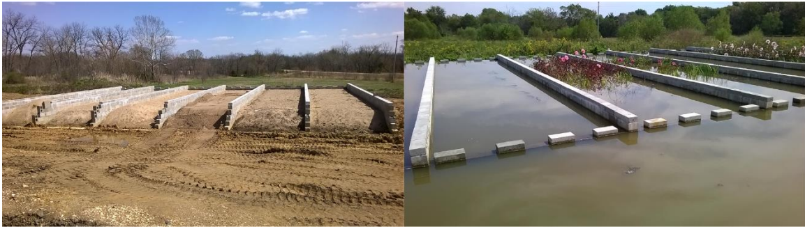
Figure 2.2 - Cells with different media mixes and that either contained plants or did not contain plants.
