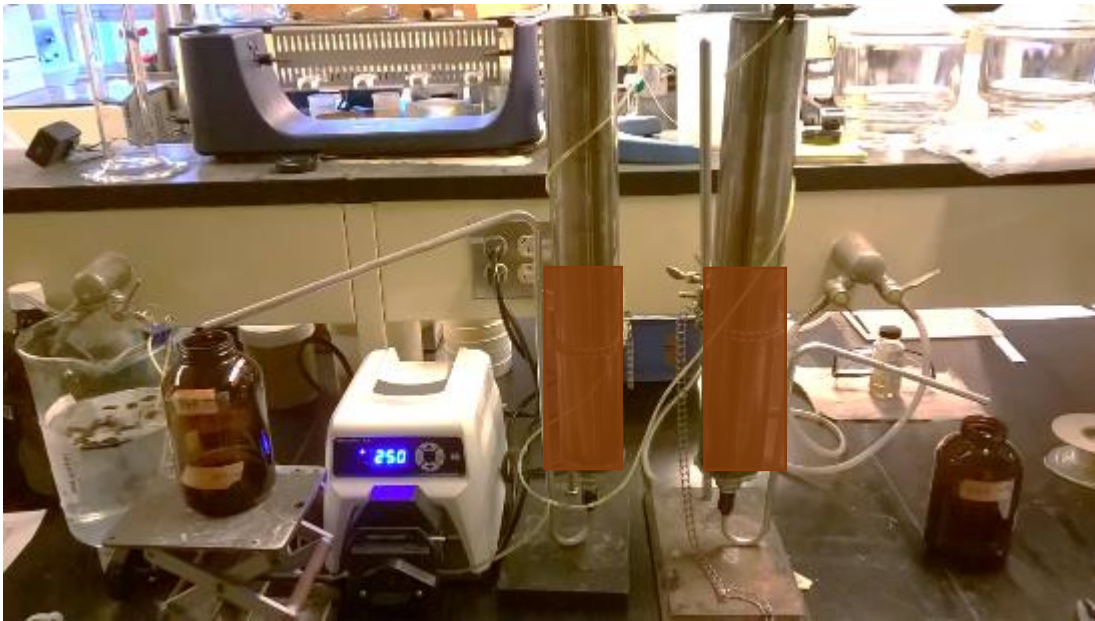
Figure 3.1 - Experimental setup. Saturated column is on left, partially saturated column is on right. Shading approximates media surface.
