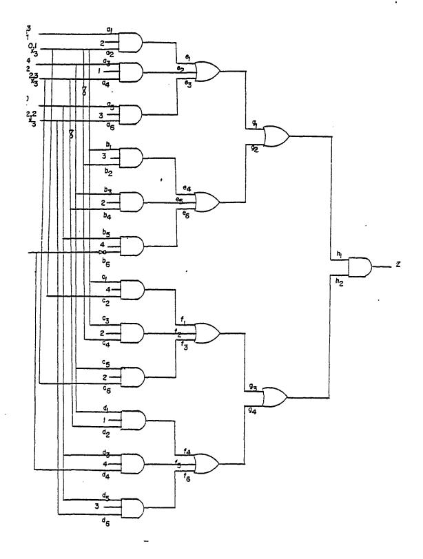
Figure 7.3.4: Circuit of Example 7.3.2
