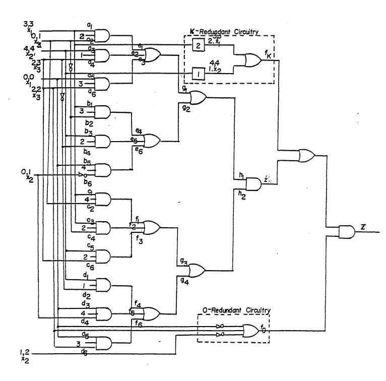
Figure 7.3.8: Static hazards free circuit of circuit of Figure 7.3.4.
