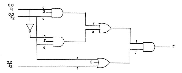
Figure 7.3.1: Circuit of Example 7.3.1.
