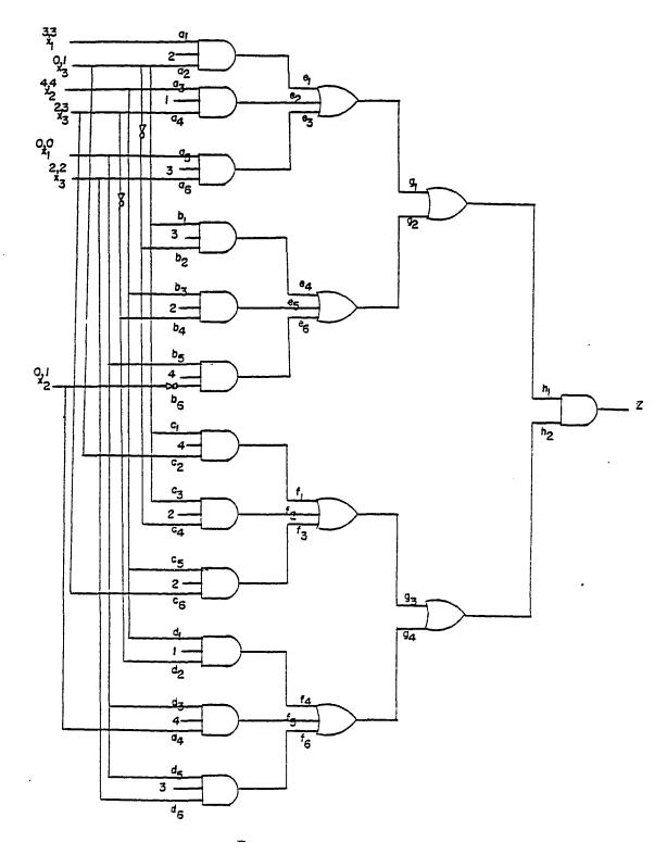
Figure 6.5.4: Circuit of Example 6.5.3
