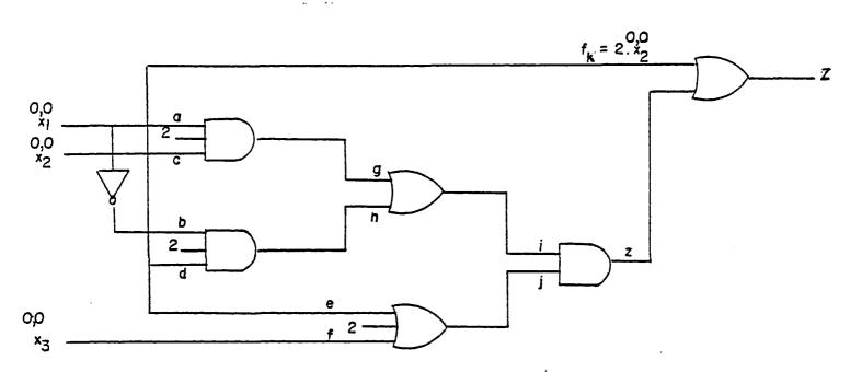
Figure 7.3.3: Static hazards free circuit of circuit of Figure 7.3.3.
