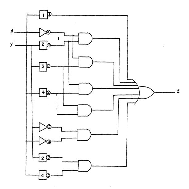
Figure 3.2.6: AND-OR Realization of Equation (3.2.19).
