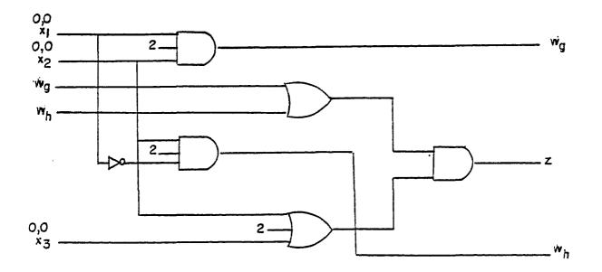
Figure 6.5.3: The circuit of Figure 6.5.1 without parallel paths.
