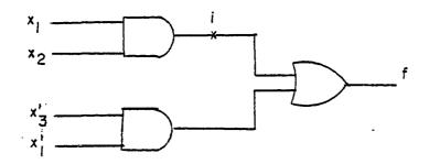
Figure 2.7.1: The Logic Circuit of Example 2.7.1
