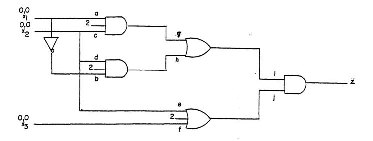
Figure 6.5.1: Circuit of Example 6.5.1.
