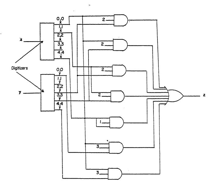
Figure 3.2.3: K-AND-OR Realization of Equation (3.2.10).
