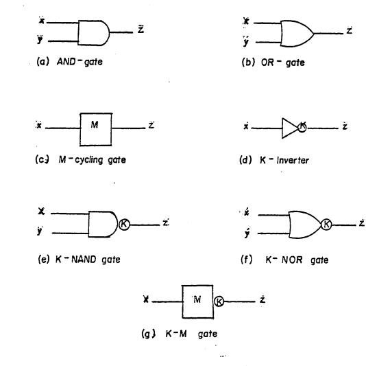
Figure 3.2.5: Seven basic gates of the multi-valued switching system derived from algebra B.
