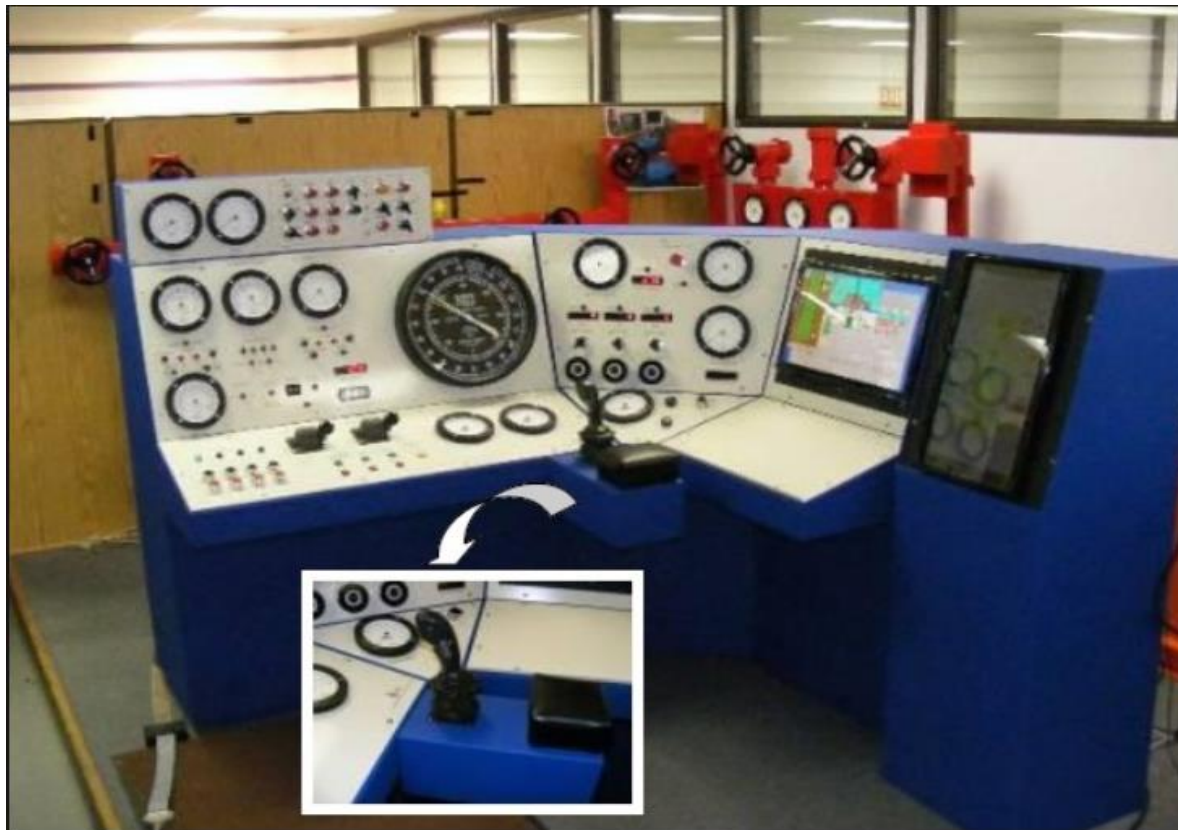
Figure 43: Typical hardware drilling rig control panel [40].
