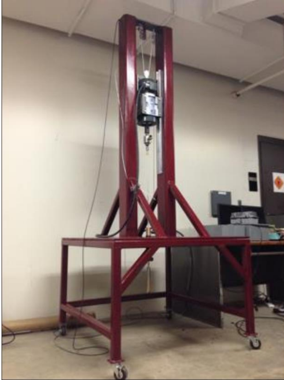
Figure 21: Texas A&M University drilling rig setup [28].
