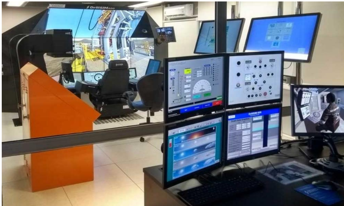
Figure 44: Simulator systems of Drilling Systems used by Pan American Energy [39].
