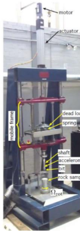
Figure 15. Apparatus used by Kovalyshen [8].
