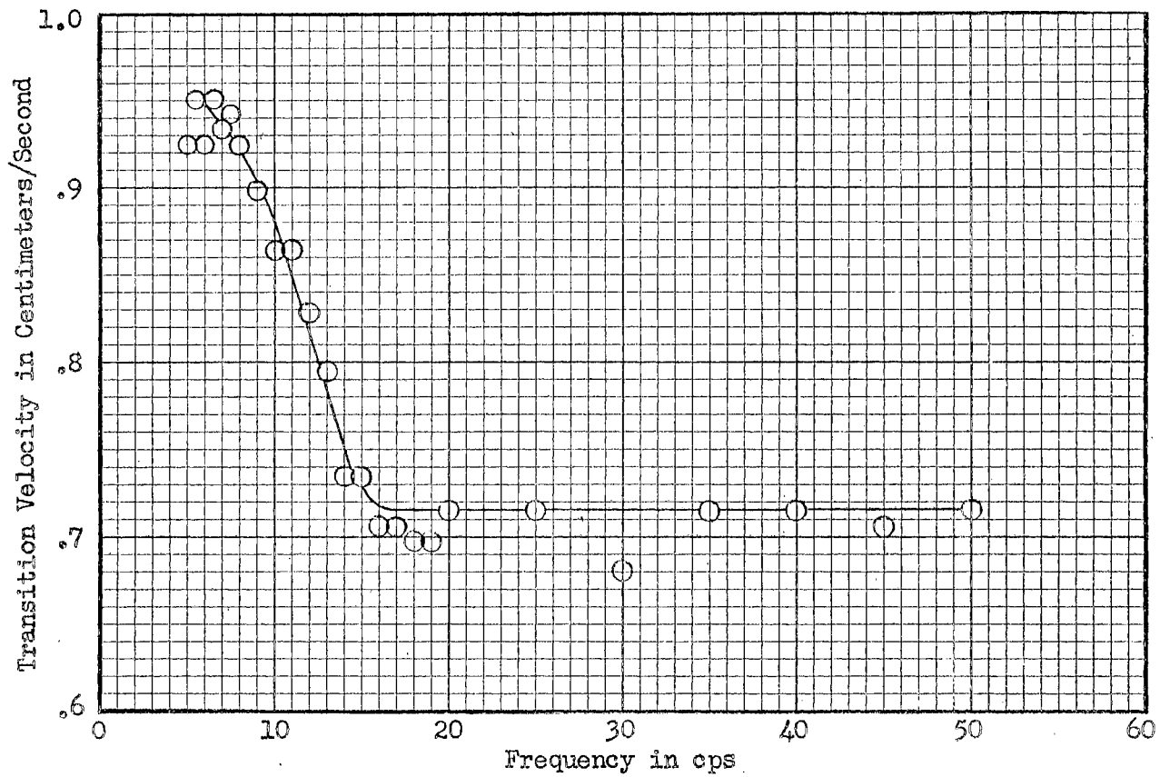
Figure 16. The plane velocity amplitude at which the transition from pattern (d) to (e) as shown in figure 7 occurs as a function of frequency of oscillation for a 2.56 cm plane in a 1.30% milling yellow solution. The observed plane velocity is positive maximum.
