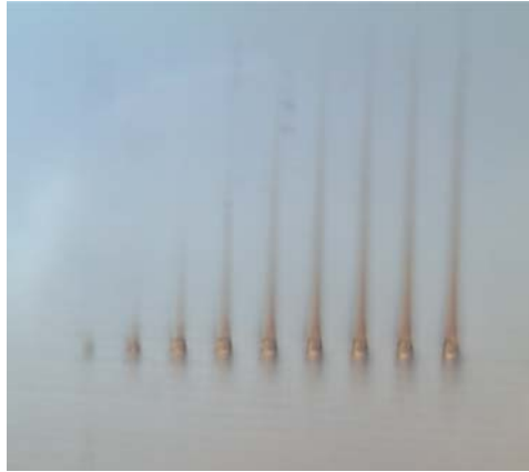
Figure 5-9. DIC image of matrix of waveguides written with varying pulse energy and Z_0=40\mu\text{m} .
