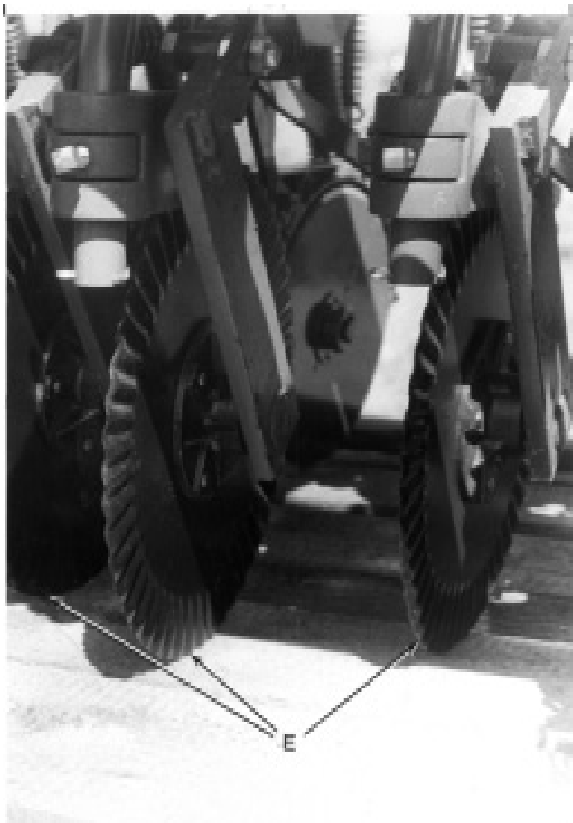
Figure 3. Specially modified drills are preferred for planting grasses. Desirable features include (a) double-disc openers, (b) depth bands, (c) press wheels, (d) large drop tubes, (e) cutting coulters, and (f) seedbox agitators.
