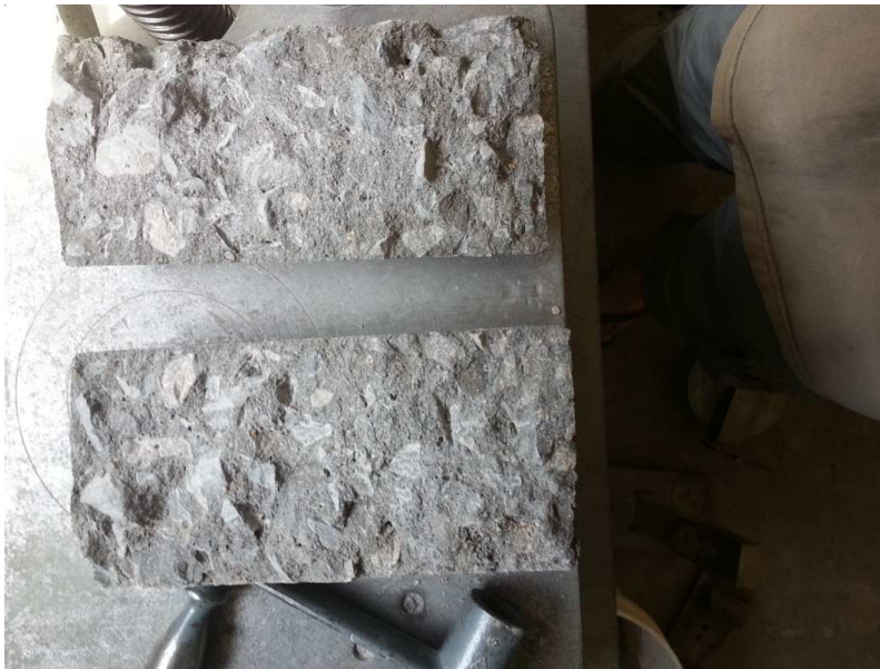
Figure 25 Splitting Tensile Strength vs. Time according to ASTM C496, Mean 28 days tensile strength was 570 psi which is approximately 9% of the 28 days compressive strength.
