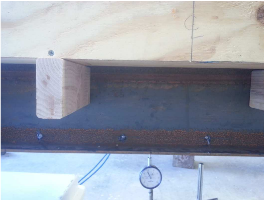
Figure 21 Shows DEMEC points glued on the surface of the web at 1.75 inches from the bottom flange of prototype beam A
