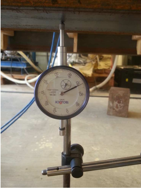
Figure 22 Shows gages for measuring changes in beams deflection at mid-span. The gages are accurate to 0.001 in.
