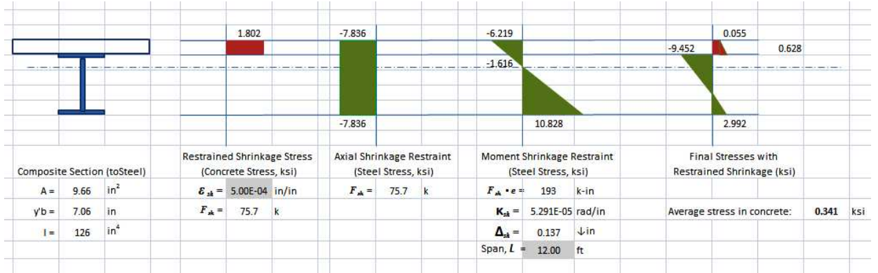
Figure 10: Stresses due to restrained shrinkage in concrete deck slab of Prototype beam #1 proportioned to resemble the SH86 Bridge
