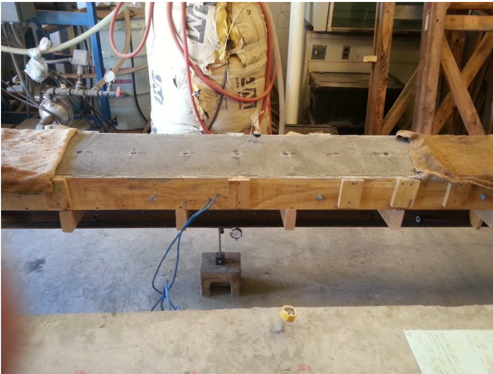
Figure 16 Deflection gage at mid-span to measure deflection
