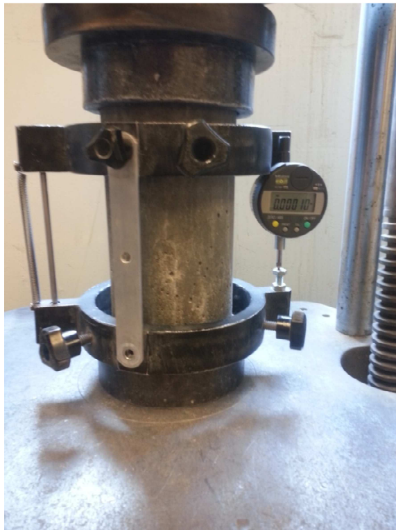
Figure 6 Set up of the elastic modulus test
