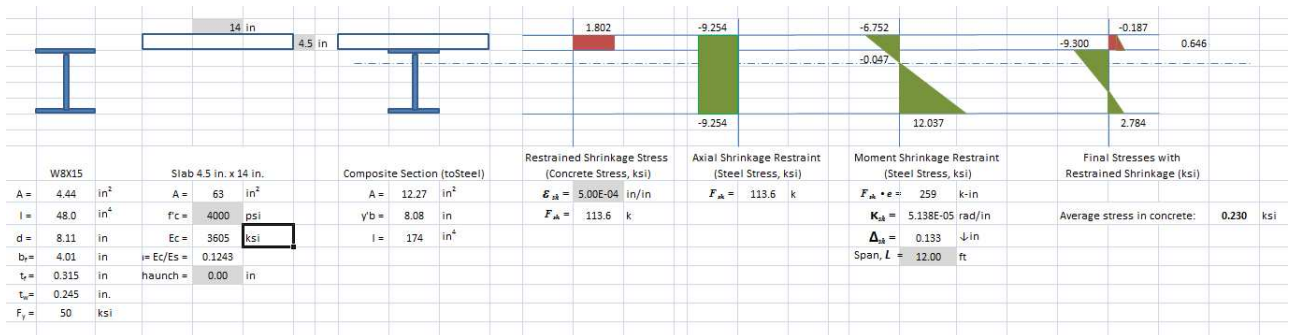
Figure 11 Stresses due to restrained shrinkage in concrete deck slab of Prototype beam #2 proportioned to resemble the SH86 Bridge
