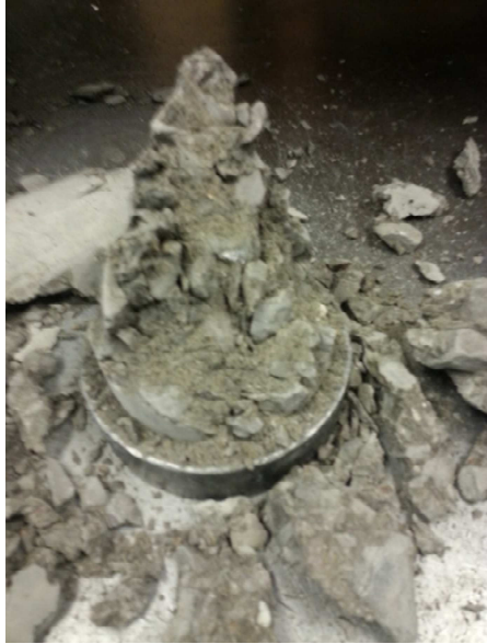
Figure 5 Type 1 failure (cone failure)
