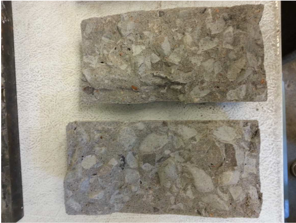
Figure 27 Tensile Split Failure - 7 Days - Slab 2, failure starts to take place more in aggregates.
