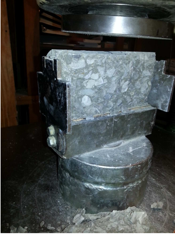
Figure 7 Split tensile failure
