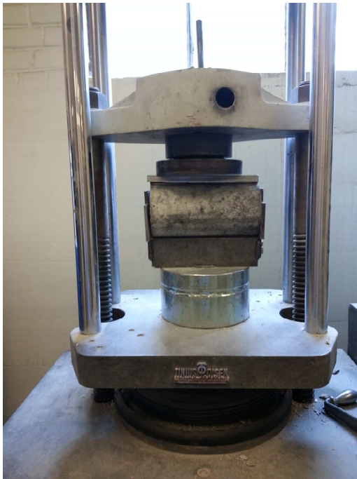
Figure 8 The setup of the splitting tensile strength test
