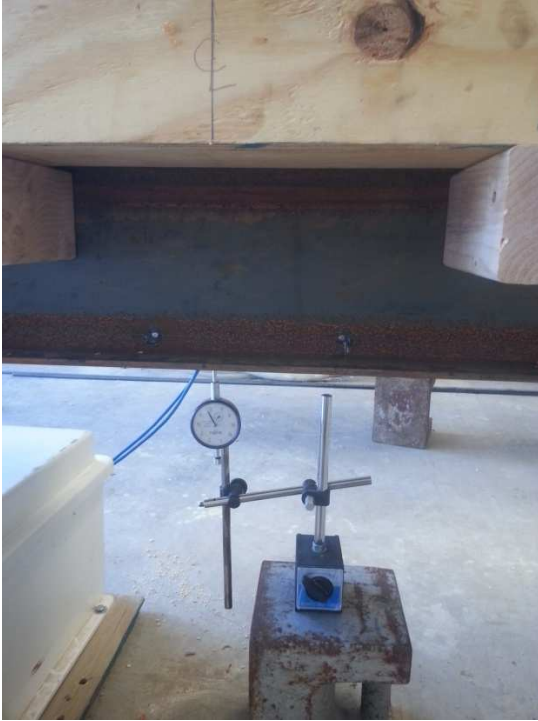
Figure 13 Deflection gage set up at the midspan of the beam.
