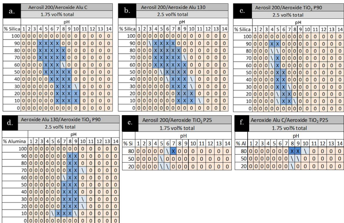
Figure 10. Phase behavior diagrams for various binary mixtures of fumed metal oxide nanoparticles in deionized water. X's indicate gel formation, O's indicate low-viscosity suspensions, and /'s indicate mild viscosity increases. Both silica/ alumina mixtures (a&b) experience gelation in a pH range between 4 and 10 with the gel region shifting to higher pH range as Si/ Al ratio decreases. Silica/ titania mixtures (c&e) show gelation between pH's 4 and 7, and alumina/ titania mixtures show gelation between 7 and 9. For different alumina and titania particles tested, the particles with smaller primary particle size (Alu130, Ti P90) were more effective for gel formation.
