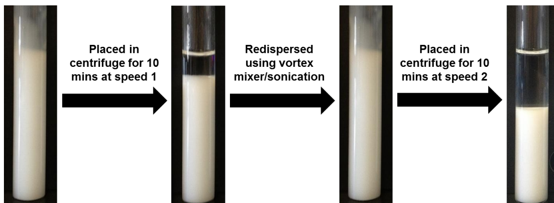
Figure 27. Method used to study gel stability against sedimentation
