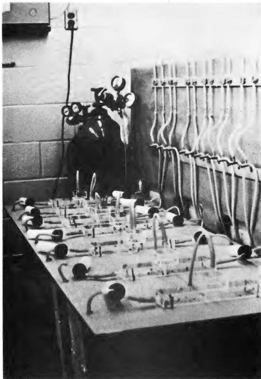
Figure 4. The appearance of the olfactometer system during tests.
