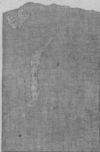
FIG. 15. Southwest side of a pit at North Star mine, Portland East, Ottawa County, Quebec, Canada. A, apatite; B, pyroxene. Scale: 1 inch = 10 feet.
