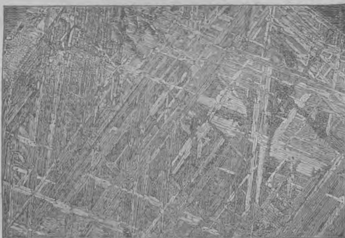
FIG. 5. Etched surface of Grand Rapids meteorite.
