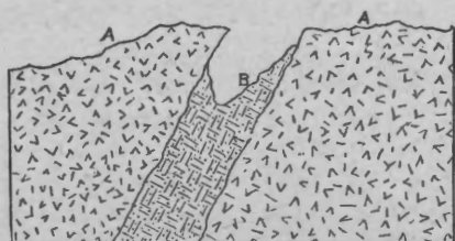
FIG. 7. Section of apatite vein near Smith's mine, Oso, Frontenac County, Ontario, Canada. A., country syenite; B, red and green apatite. Scale: 1 inch = 8 feet.
