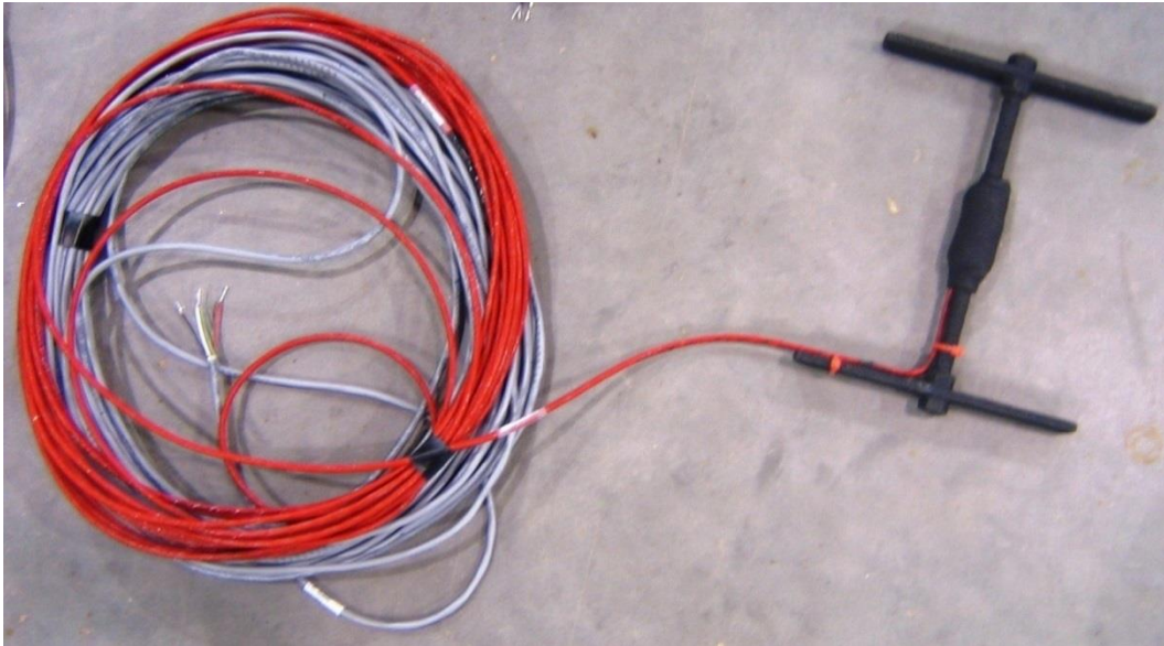
Figure 3-18 CTL Asphalt Strain Gauge
