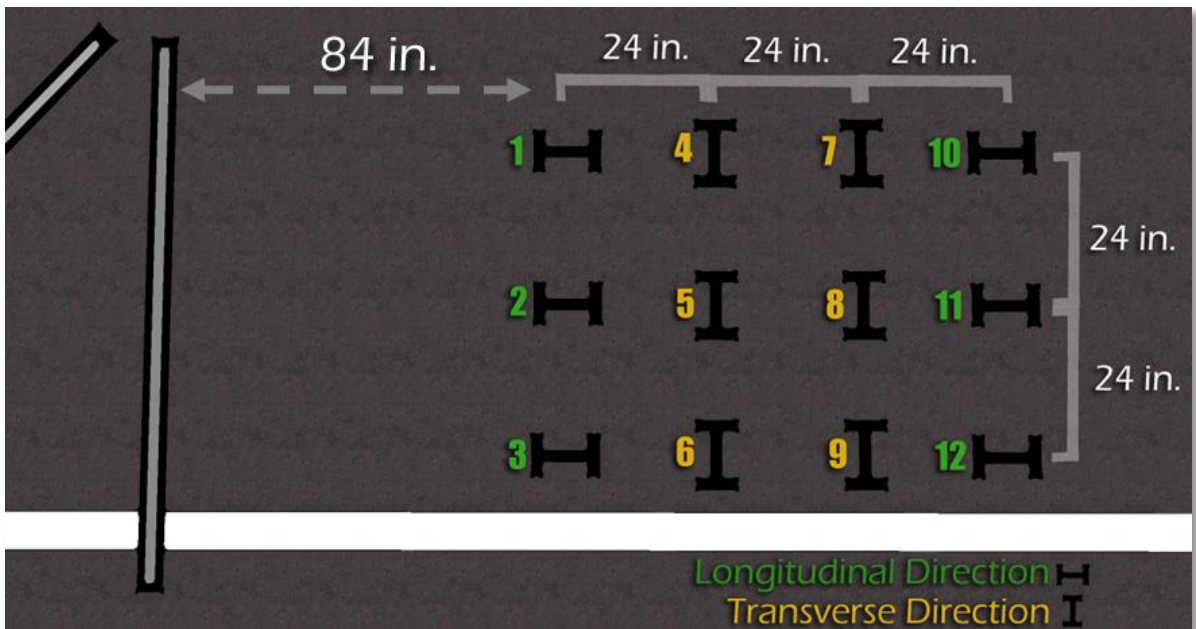
Figure 3-35 Layout of Strain Gauges
