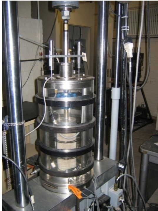
Figure 3-5 Setup for Resilient Modulus Testing on Subgrade Soil Specimen
