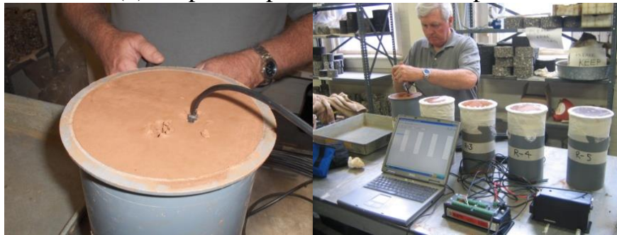
(c) ECH2O EC-5 While Taking Readings Figure 3-28 Calibration of Moisture Probes
