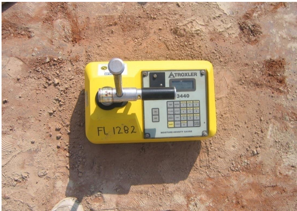
Figure 3-51 Measuring Moisture Content and Dry Density using a Nuclear Density Gauge
