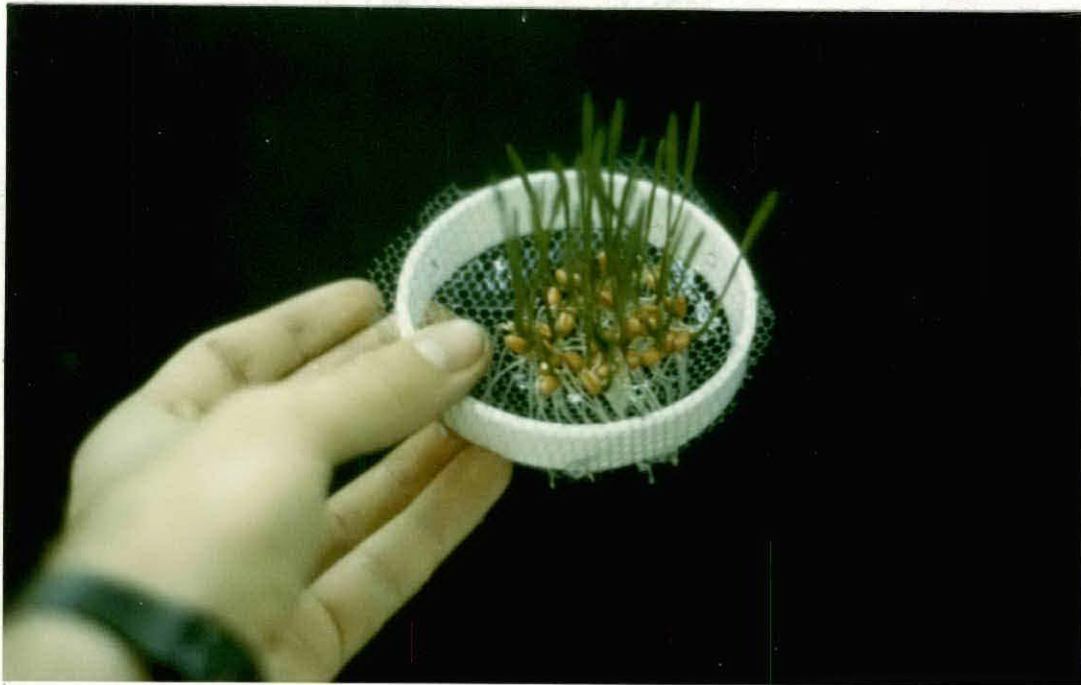
Figure 1. Net ring for hydroponic growth of wheat seedlings. The poly-styrofoam ring was cut from the top of disposable coffee cups; the nylon net was purchased at a local fabric store, as were the stainless steel pins used for holding the net in place (non-stainless steel pins rusted in the acidic environment).
