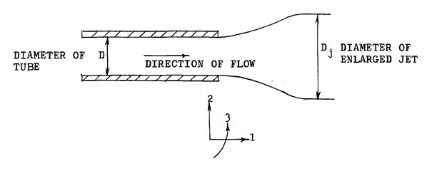
FIGURE 5-5. FLOW OF A VISCOELASTIC FLUID OUT OF A CAPILLARY
