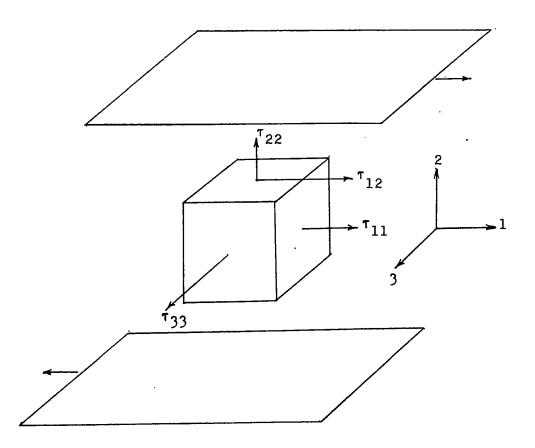
FIGURE 3-1. SHEAR DIAGRAM
