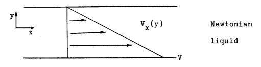
FIGURE 2-2. STEADY LAMINAR VELOCITY PROFILE FOR A NEWTONIAN FLUID CONTAINED BETWEEN TWO PLATES.
