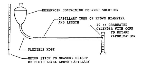
FIGURE 4-3. DIAGRAM OF CAPILLARY VISCOMETER and length of capillary. The shear rate and shear stress are then calculated by means of Equations (3-8) and (3-9), and the viscosity by Equation (3-11). The reservoir containing the polymer solution was arranged so that it could be moved up or down. The pressure drop,  $\Delta P$ , across the capillary is
