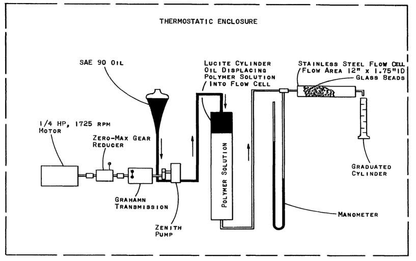
FIGURE 472. APPARATUS FOR THE FLOW OF FLUIDS THROUGH POROUS MEDIA
