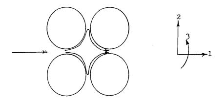
FIGURE 5-6. FLOW OF A VISCOELASTIC FLUID THROUGH A PORE
