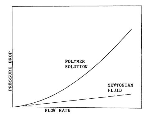
FIGURE 5-4. TYPICAL SHAPE OF A PRESSURE DROP -FLOW RATE CURVE
