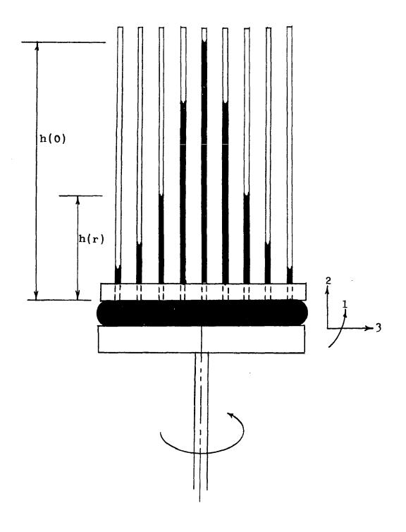
FIGURE 3-2. SCHEMATIC DIAGRAM OF PARALLEL PLATE INSTRUMENT
