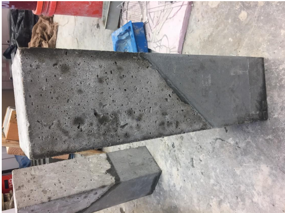
Figure 94. Composite MOR specimen prior to testing
