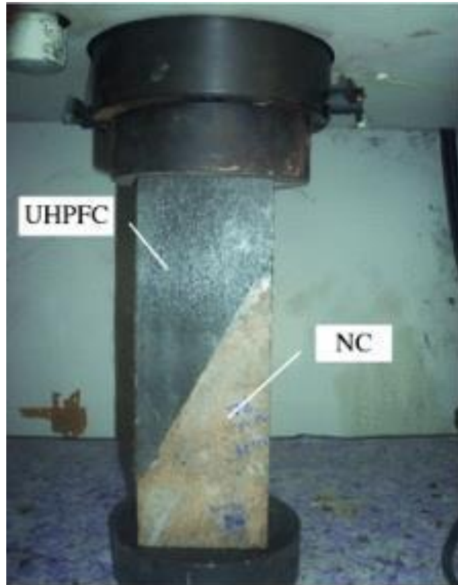
Figure 4. Prismatic specimen and testing setup for Tayeh et al. (2013) experiments
