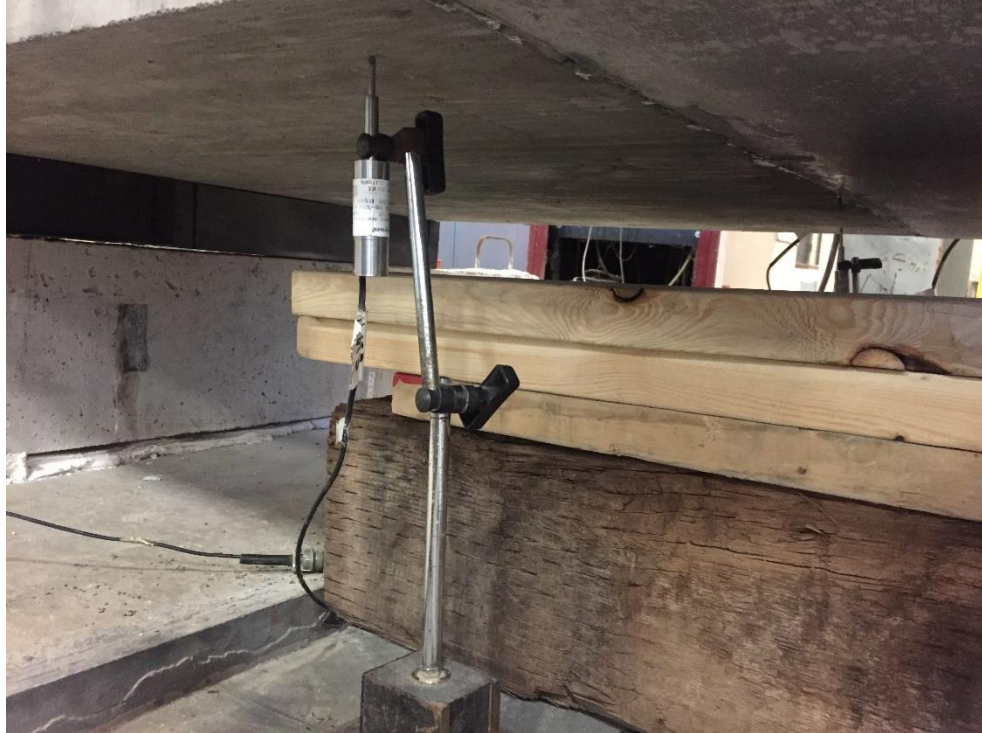
Figure 99. LVDT on underside of slab prior to testing
