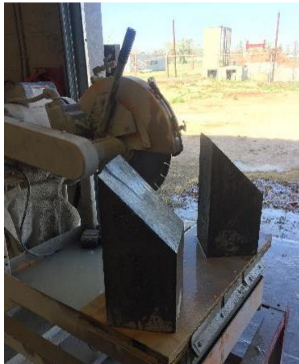
Figure 11. 45 degree specimen immediately after cutting
