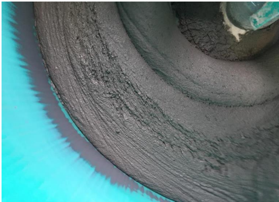
Figure 20. Final consistency of UHPC mixture prior to adding steel fibers
