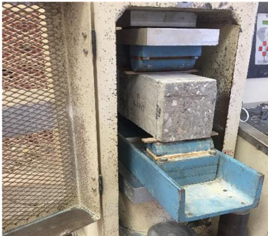
Figure 23. Testing setup for composite MOR specimens
