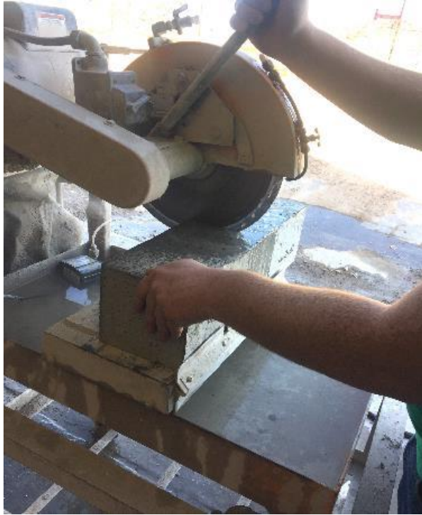
Figure 10. Concrete table saw used to cut MOR specimens
