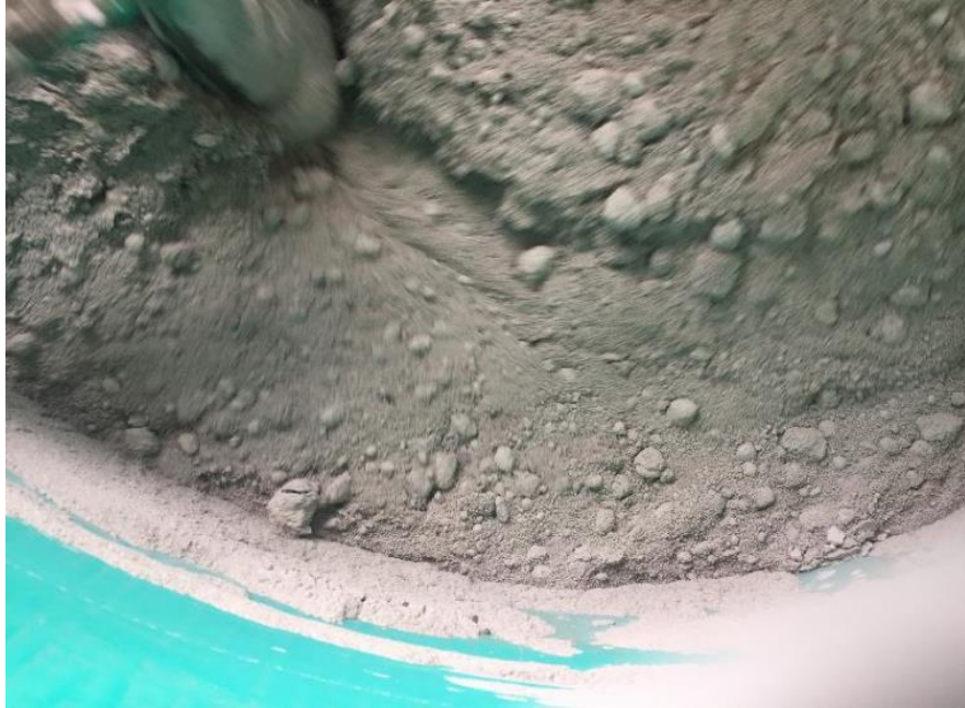
Figure 17. Beginning stages of mixing after water was added to dry premix
