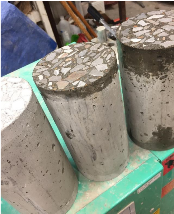
Figure 90. NSC cylinders after grinding prior to compressive strength testing
