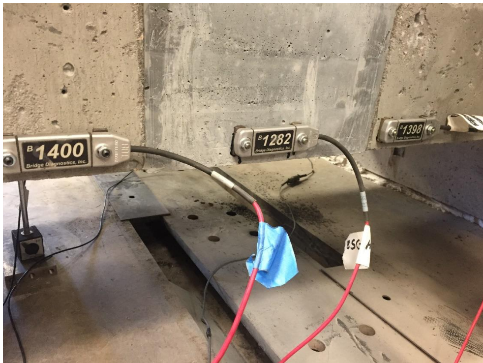
Figure 98. Strain gages on south side of slab prior to testing
