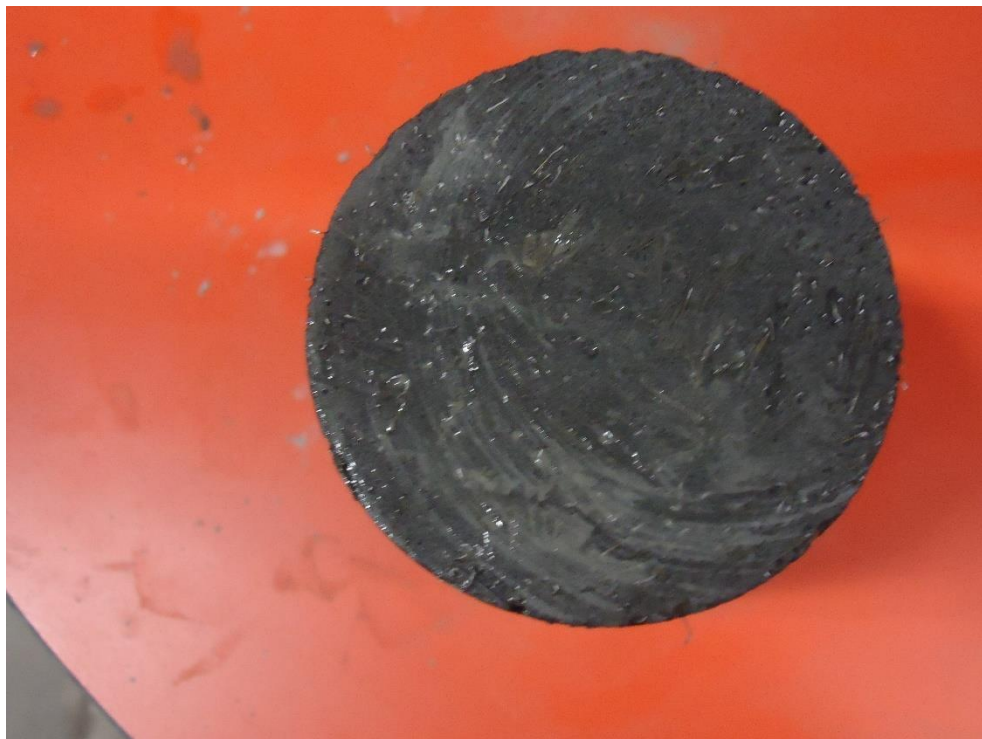
Figure 92. Top surface of UHPC cylinder after grinding prior to compressive strength testing
