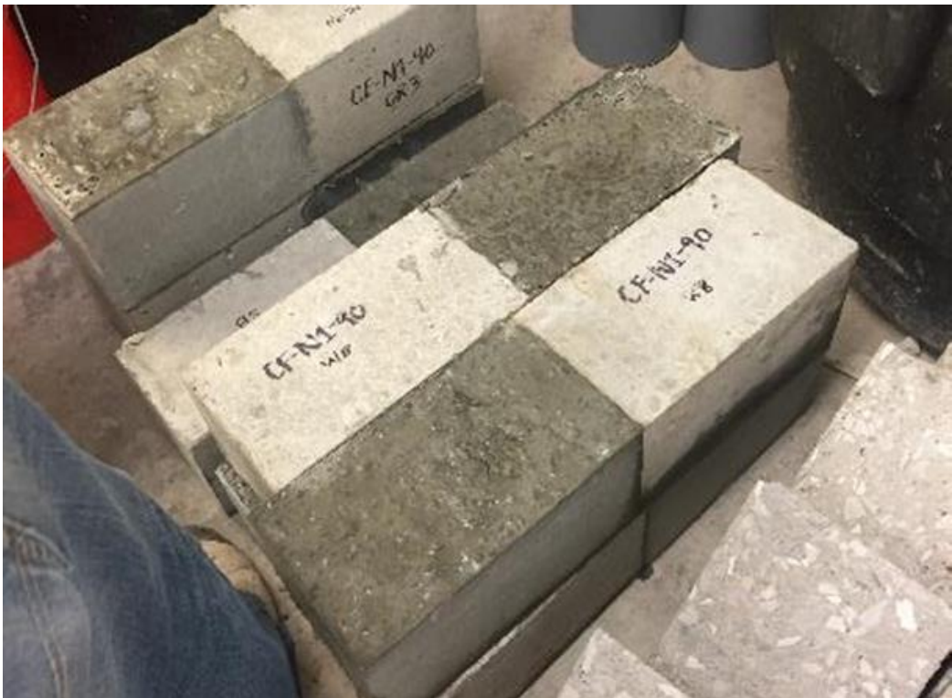
Figure 22. Composite specimens after curing
