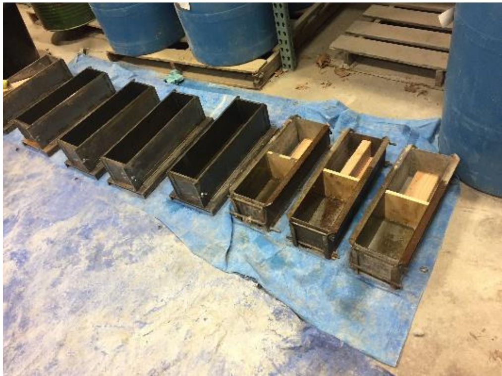
Figure 9. Layout of formwork ready for concrete to be cast. From left to right: two for sandblasted specimens, two for wire-brushed specimens, and three for exposed aggregate specimens
