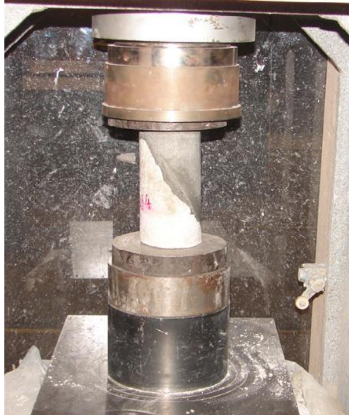
Figure 5. Cylindrical specimen and testing setup for Sarkar (2010) experiments
