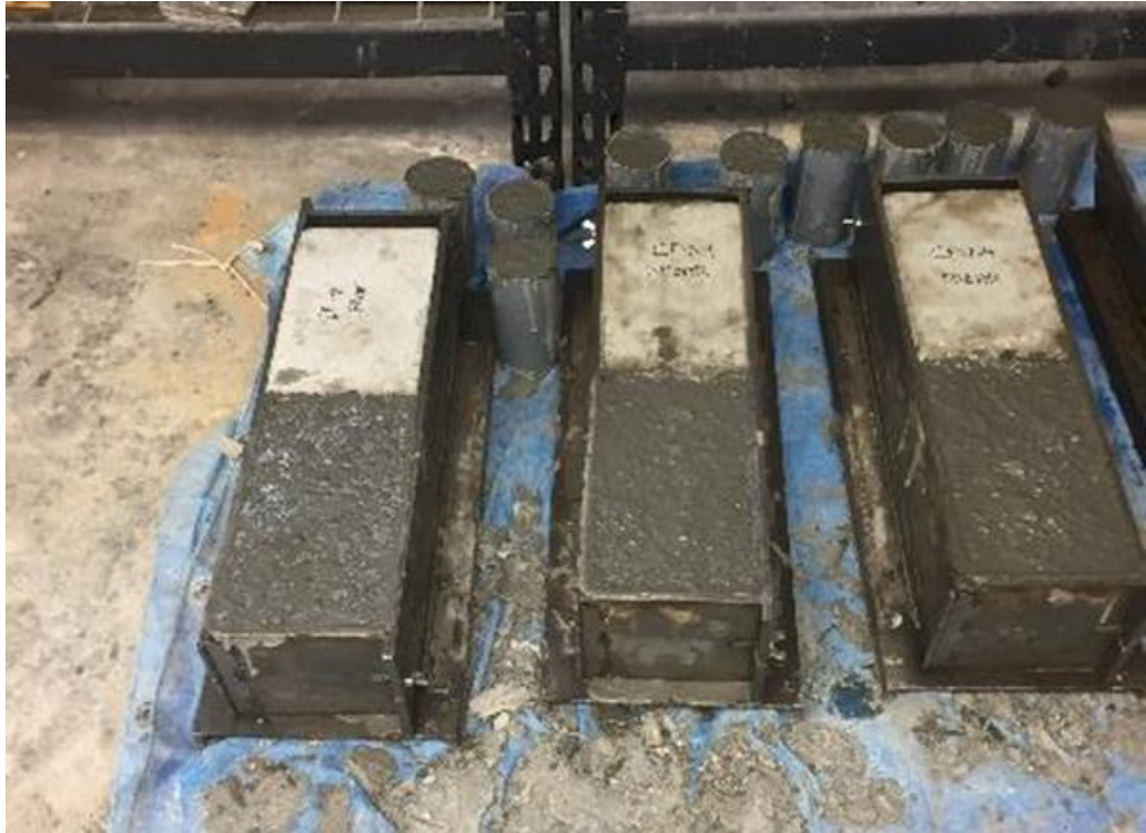
Figure 21. Composite specimens immediately after casting
