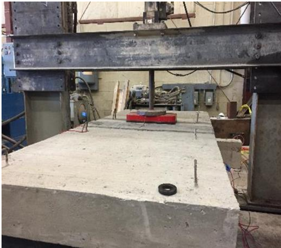
Figure 31. Testing setup for slabs
