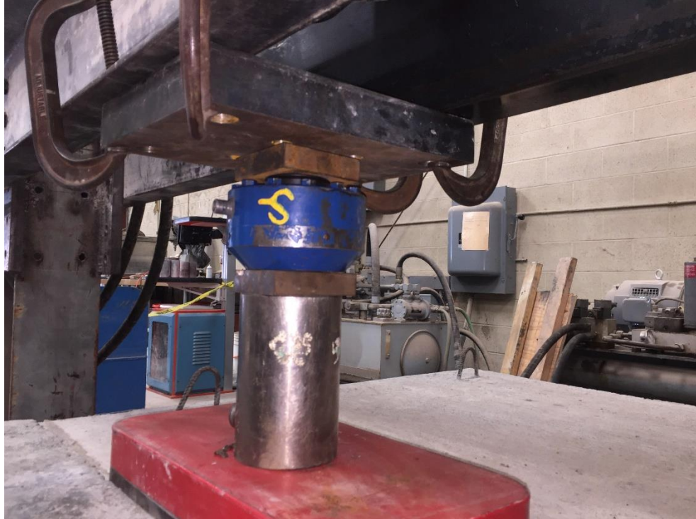
Figure 101. Hydraulic cylinder and load cell prior to attachment to hand pump; used for part 2 of static testing
