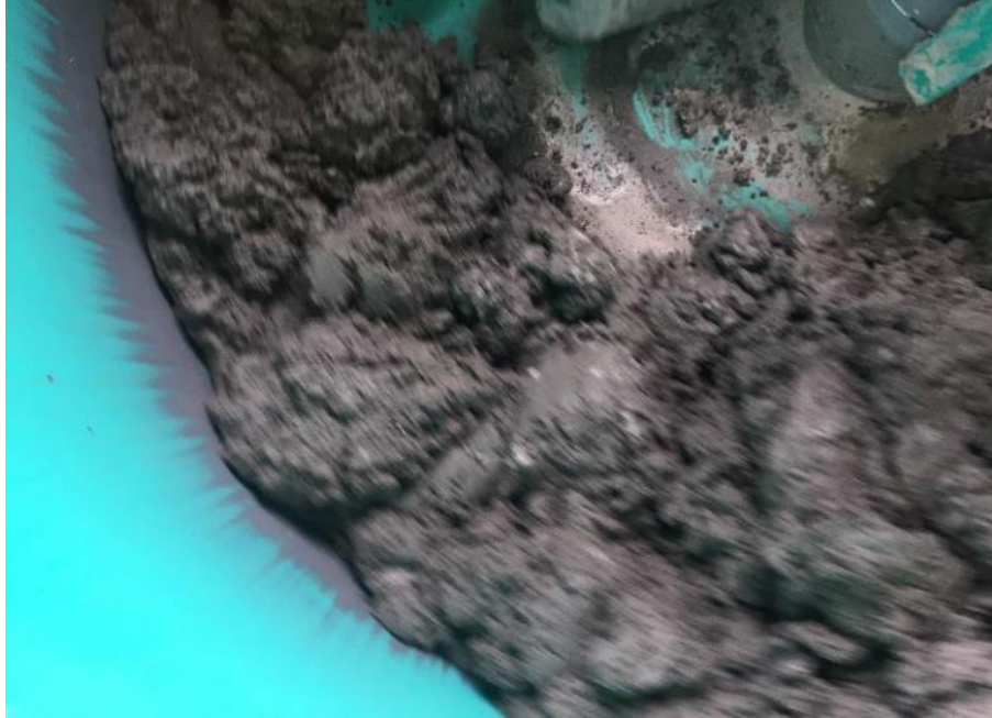
Figure 19. Consistency after several minutes of mixing beyond final addition of high-range water reducer, no additional components were added to reach this point
