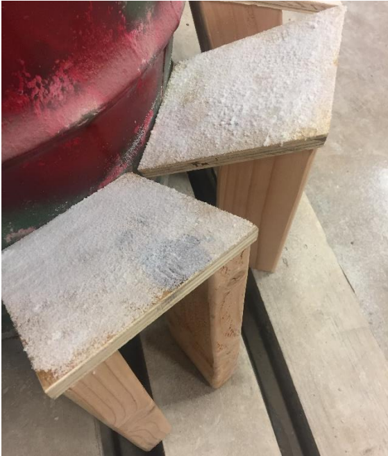
Figure 89. Wooden MOR form inserts coated with sugar for exposed aggregate specimens
