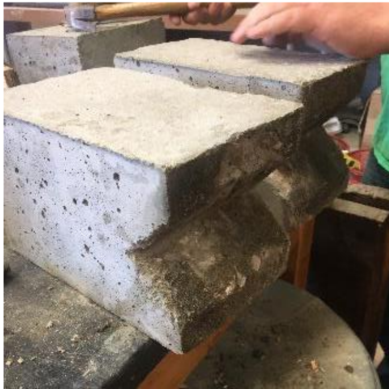
Figure 14. Shear key specimen after being de-molded
