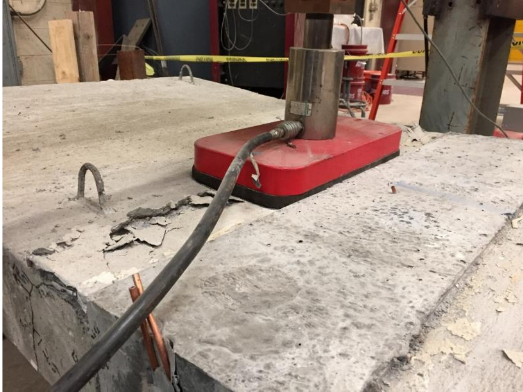
Figure 86. Crushing of concrete on top of slab after final static loading
