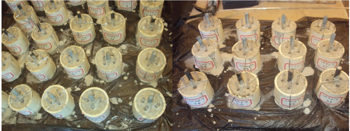
Figure 3.14 Prepared cylindrical concrete samples with embedded rebar
