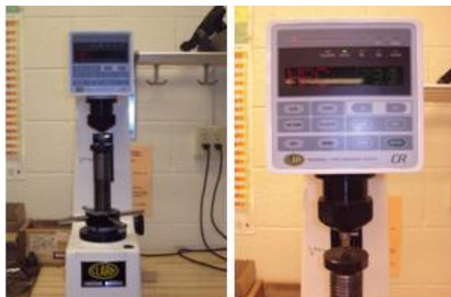
Figure 3.4 CLARK CR Series Rockwell hardness tester
