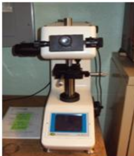
Figure 3.7 Clark model CM-400AT Vickers hardness tester
