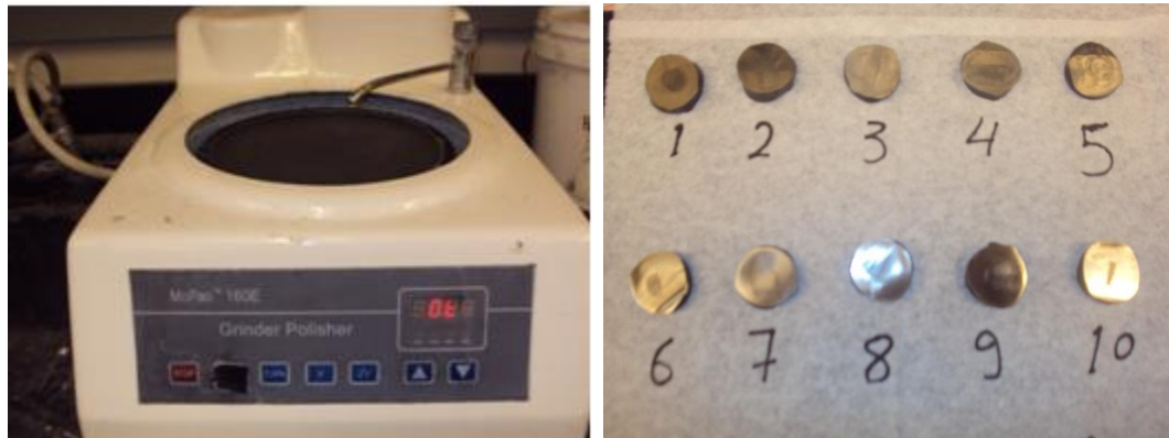
Figure 3.8 The polishing apparatus and the circular samples
