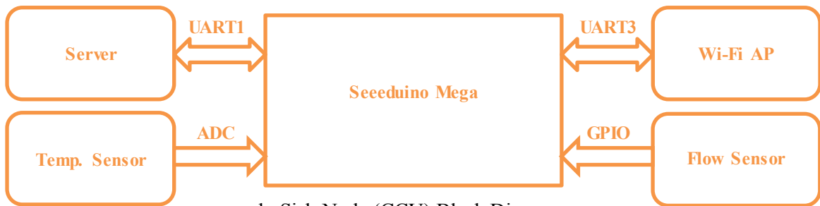
b. Sink Node (CCU) Block Diagram
