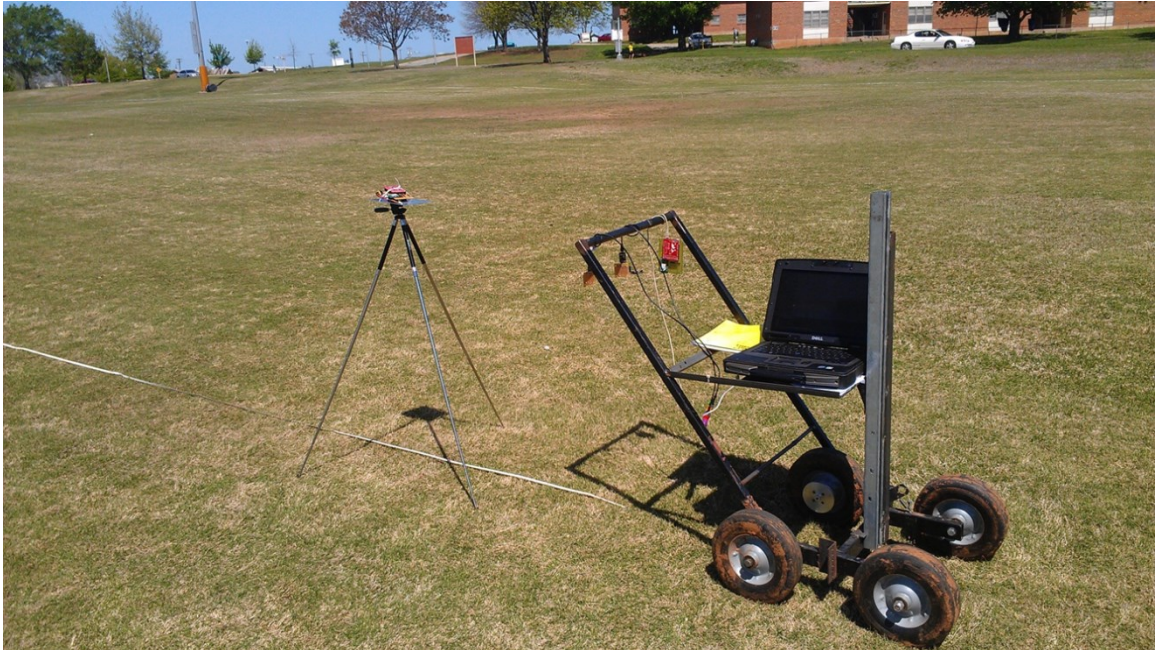
Figure 24 RSSI vs. Distance Measurement Field Test Setup
