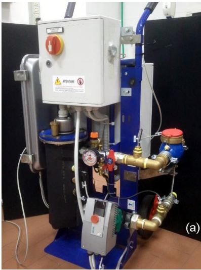
Figure 1 TRT machine developed at the University of Genova (a) and TRIAC power response vs control signal (b).
