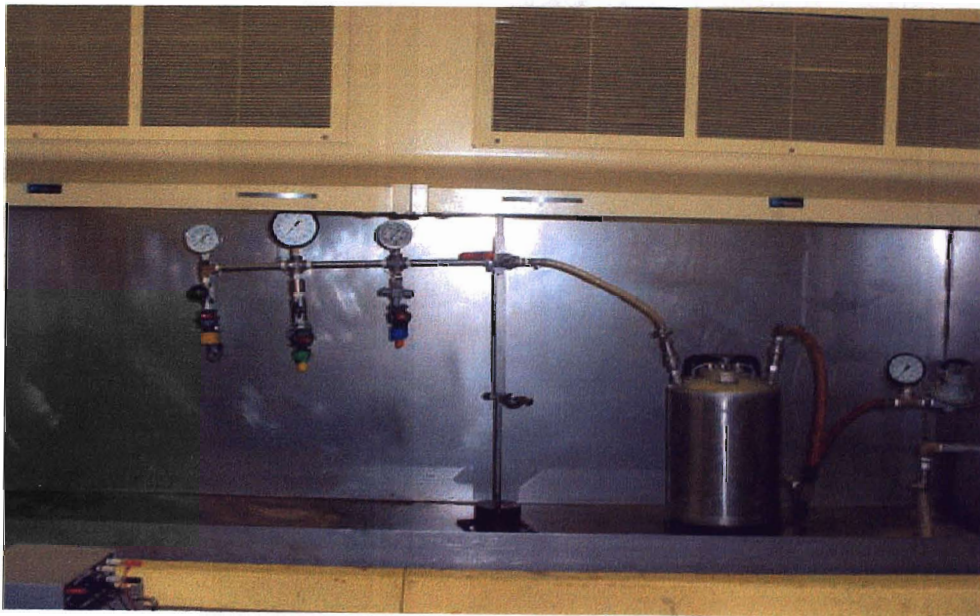
Figure 2. Test apparatus including air supply, pressure regulator, pressure gauges, Remcor solenoid valve, and nozzles.
