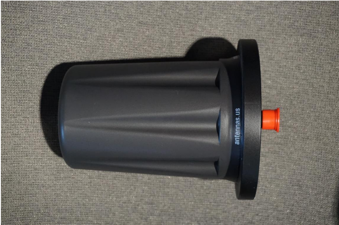
Figure 42. Broadband UL-235A-498 horn antenna for N210-based SDR testbed.
