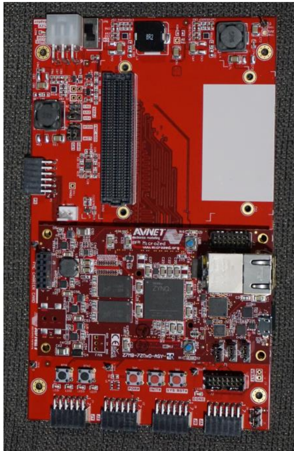
Figure 31. The MicroZed Board (top) and the MicroZed FMC Carrier (bottom)
