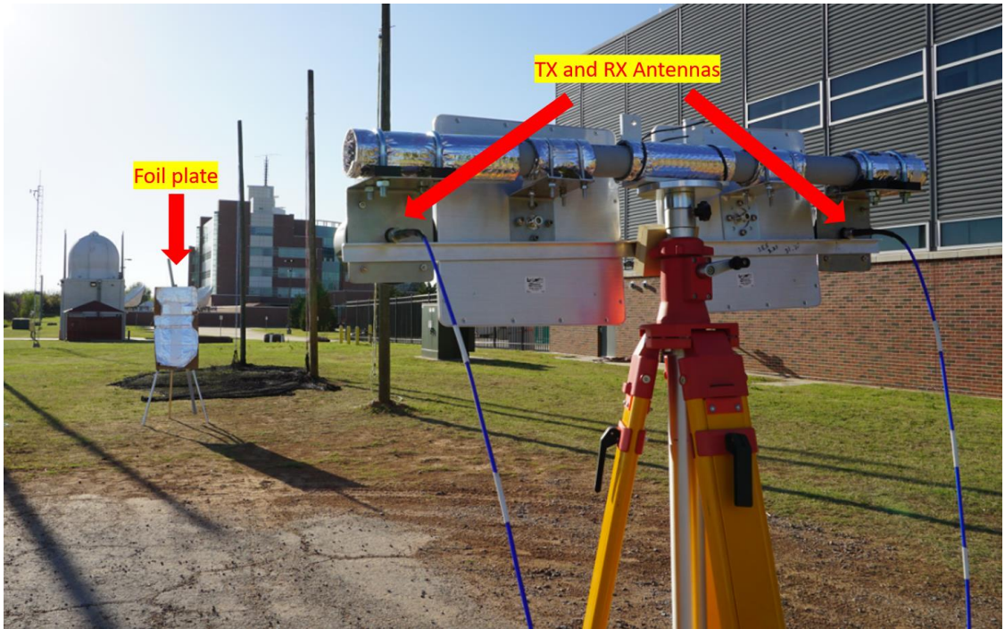
Figure 59. Outdoor experiment using N210-based SDR and a reflective plate as targets
