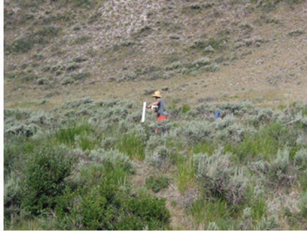
FIGURE 3: Using the handheld gradiometer in the field introduces a wide range of nonlinearity. Flora, terrain, and user inconsistencies all add to uncertainty inherent in the measurements.
