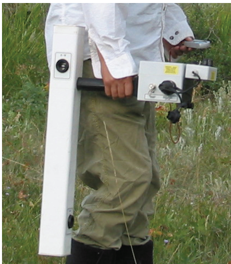
FIGURE 2: FM36 Magnetic Gradiometer by Geoscan Research (Bradford, West Yorkshire, UK). This handheld device is used to scan for subsurface archaeological features.
