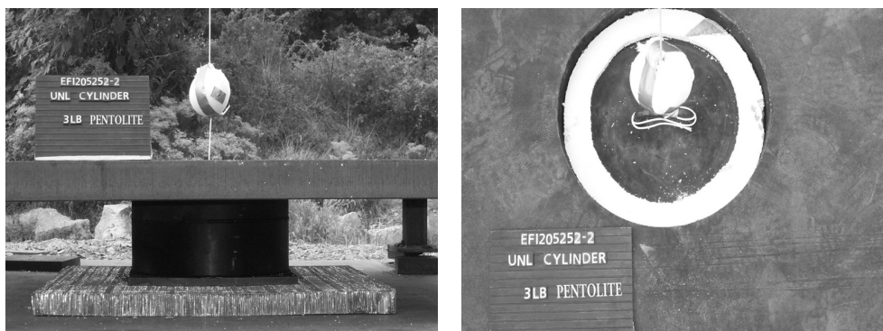
Fig. 2. The first experimental setup for the explosive charge test.
