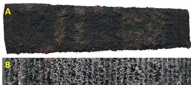
Fig. 10. Mosaicked RGB images of plant canopies from the continuous motion mode of NU-Spidercam A: The soybean canopy image mosaicked automatically with Pix4D; B: The maize canopy image mosaicked manually with Photoshop.
