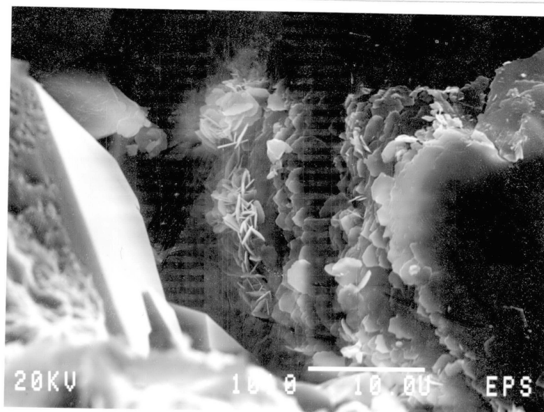
Figure 74. SEM Micrograph of Authigenic Chlorite. 2400X, Shell Bedell. Depth: 4436 ft.
