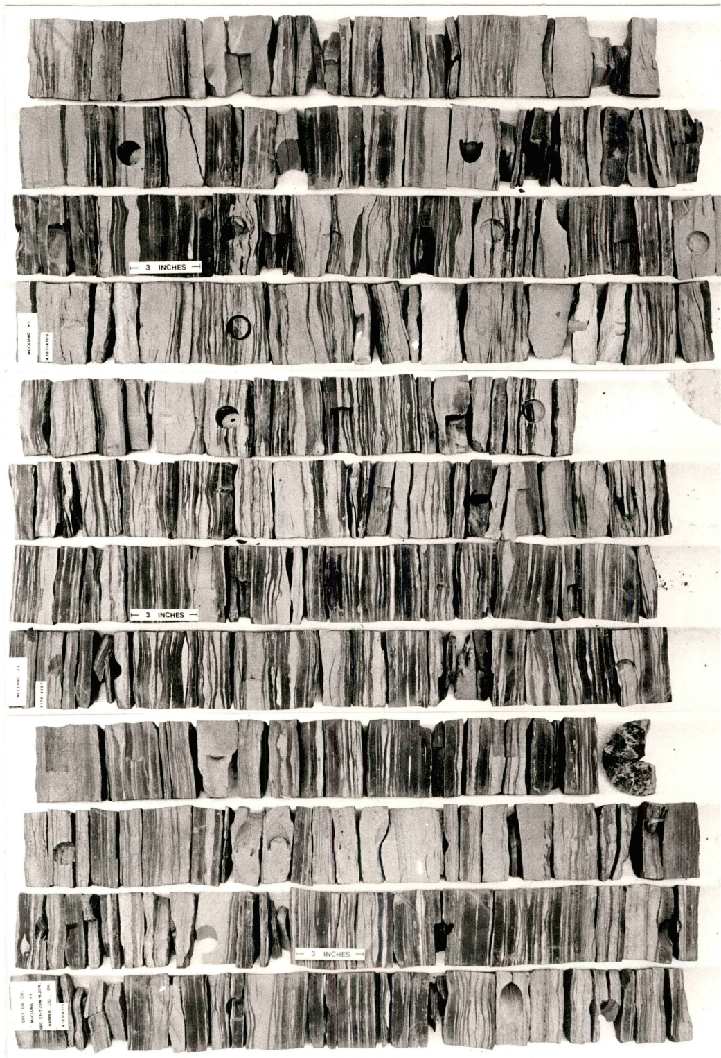
Figure 16. Photograph of Gulf McClung No. 1 Core. Depth: 4163-4199 ft.
