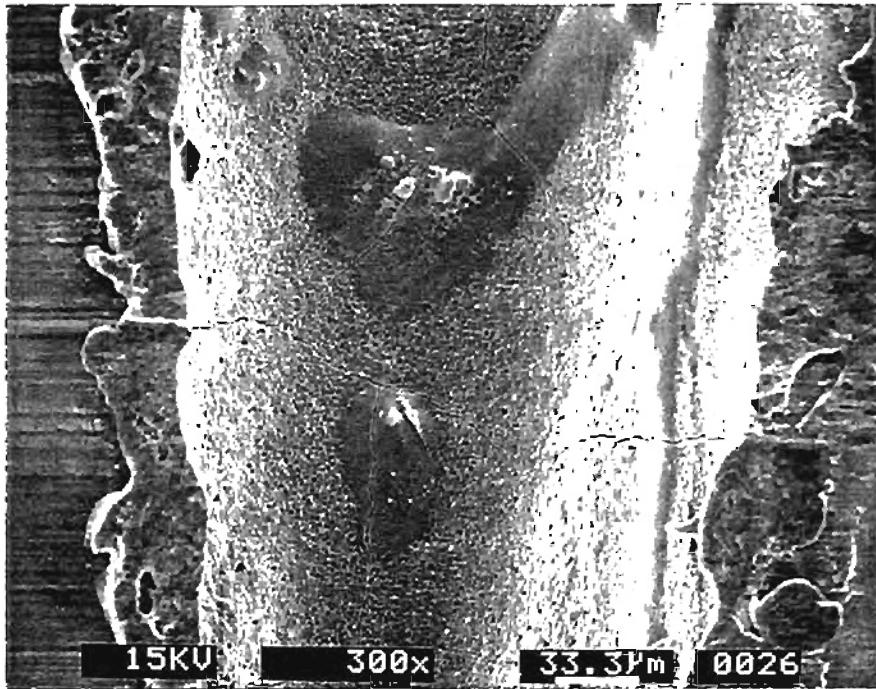
Figure 7.3.3.4 SEM Micrograph Showing Thermal Cracking in SiAlON at Low Power
