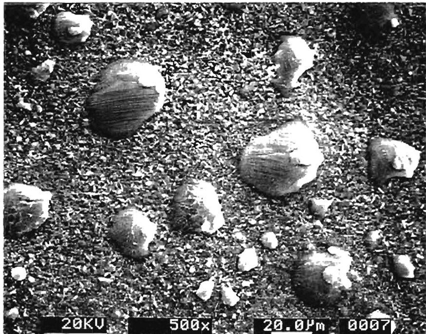
Figure 11.2.1.4 Micrograph Showing Molten Silicon in the Groove
