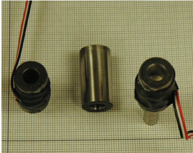
Figure 5.5: Photograph of the confinements used in the static testing of sand. The confinement (to the left) has a bonded strain gage mounted under the protective tape. The confinement (to the right) shows the compacted sand sample after test routine. The confinement (in the middle) shows a polished surface for mounting strain gage.
