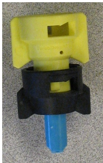
Figure 4 TurboDrop TDVR02 variable orifice nozzle (yellow) for metering with an oversized StreamJet nozzle (blue) to generate a pattern.
