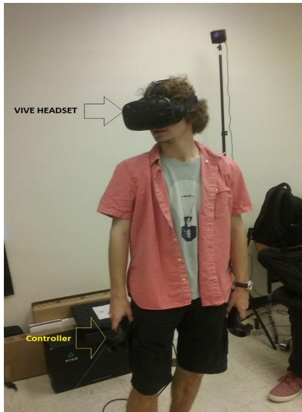
Figure 4: Fully Immersive Virtual Reality System (VIVE) with its components
