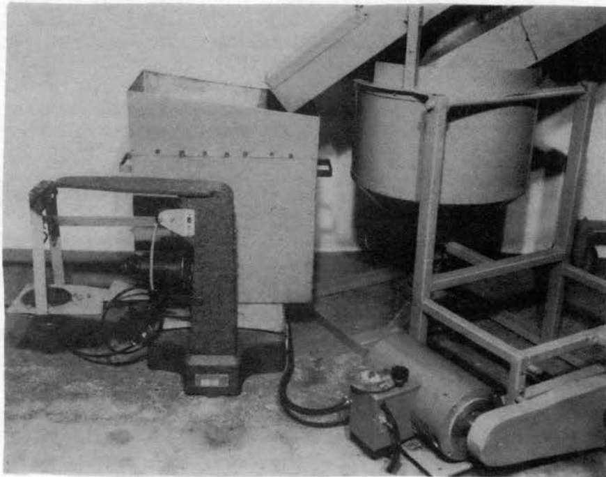
Figure 2. Platform Scale, Screw Conveyor Hopper, and Drive Mechanism
