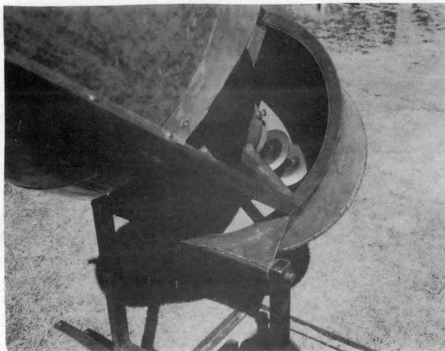
Figure 4. Conveyor Hopper With Standard Housing and Auger
