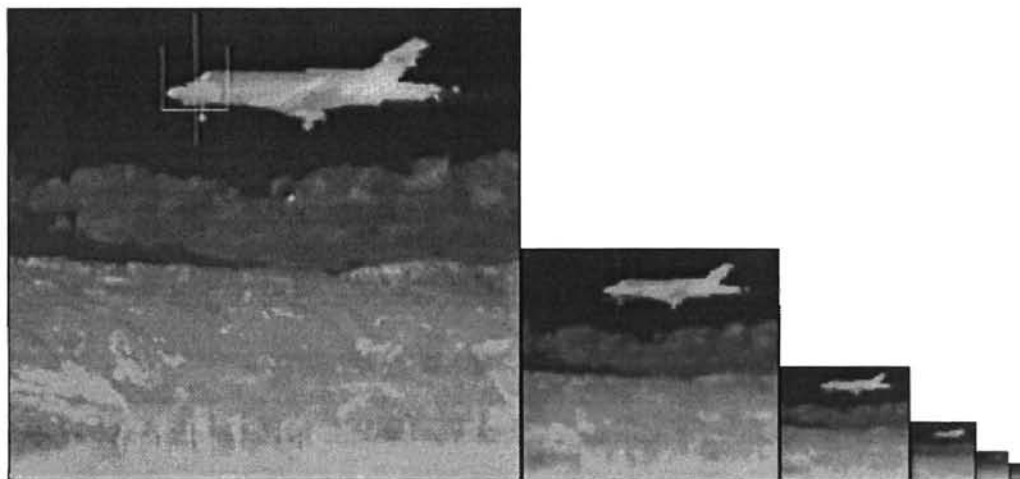
Figure 6.1 An infrared image of a jet airplane in flight and its corresponding anisotropic diffusion pyramid. The coarsest representation which contains edge features belonging to the aircraft is the fourth largest image of the pyramid (the third level).
