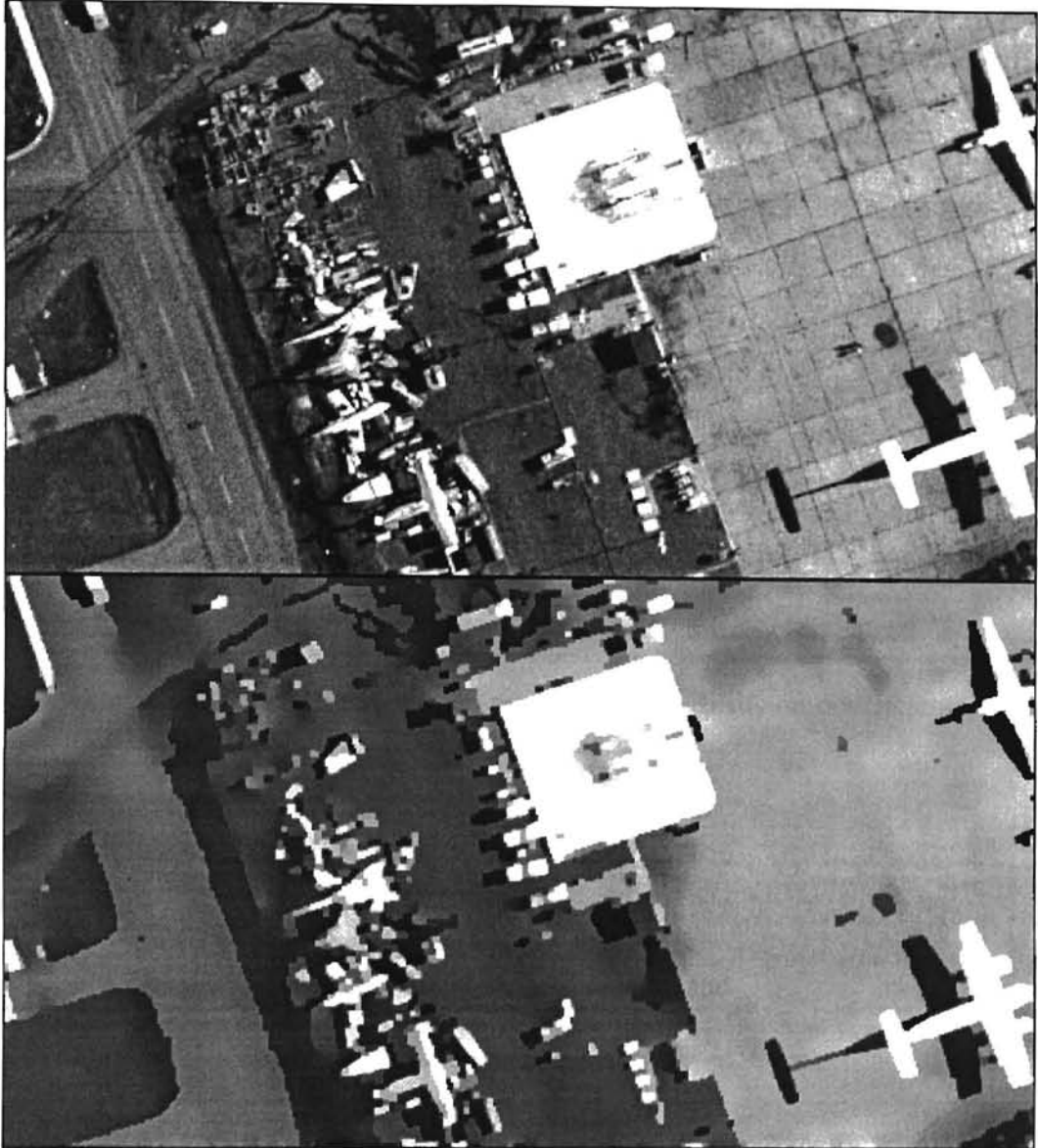
Figure 4.10 A visual example of filtering with the morphological anisotropic diffusion equation. The original image is located at the top, and its filtered result is located below. Notice how the diffusion process smooths within the boundaries of an object, preserving edge locations, but is still capable of removing objects of small spatial scale. For comparison to the other diffusion expressions, refer to Figures 2.4 and 2.7.
