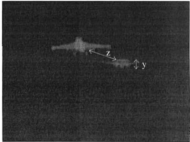
Figure 6.2 Designing a coarse to fine search that is capable of identifying the smaller aircraft in the infrared image. Root level selection is dependent on two variables, the minor axis of the target's largest feature ( y ) and the minimum distance between the target and other objects of similar or greater scale ( z ).
