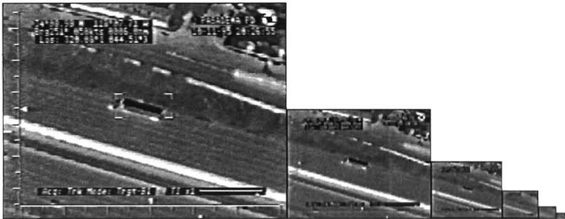
Figure 6.9 The first frame of the semi sequence and its corresponding anisotropic diffusion pyramid. The semi is visible only in the first three scene representations within the diffusion pyramid, resulting in the selection of the second level of the pyramid as the root level of the multi-scale search.
