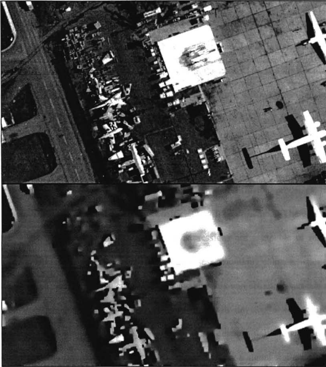
Figure 2.7 A visual example of filtering with the spatially aware anisotropic diffusion equation. The original image is located at the top, and its filtered result is located below. This diffusion process is capable of smoothing regions of small spatial size and high contrast, as evident by the removal of the small objects near the road. Spatial smoothing does reintroduce interaction across region boundaries, and this will be discussed in the next chapter.
