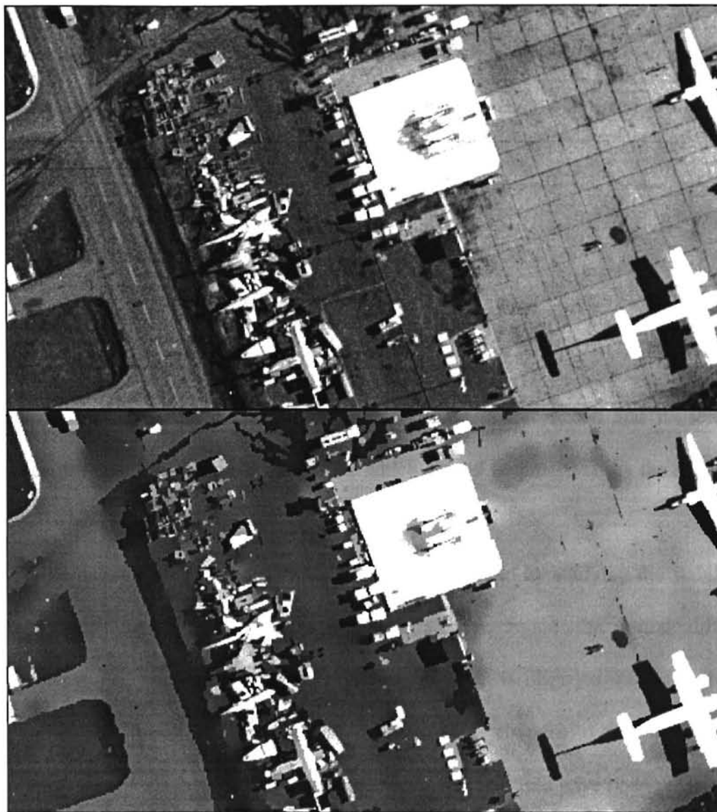
Figure 2.4 A visual example of filtering with the anisotropic diffusion equation. The original image is located at the top, and its filtered result is located below. Notice how the diffusion process smooths within the boundaries of an object but preserves the edge locations. Maintaining all features with high contrast, especially the smaller objects near the road, will motivate the exploration of spatially aware variants of the anisotropic diffusion process.
